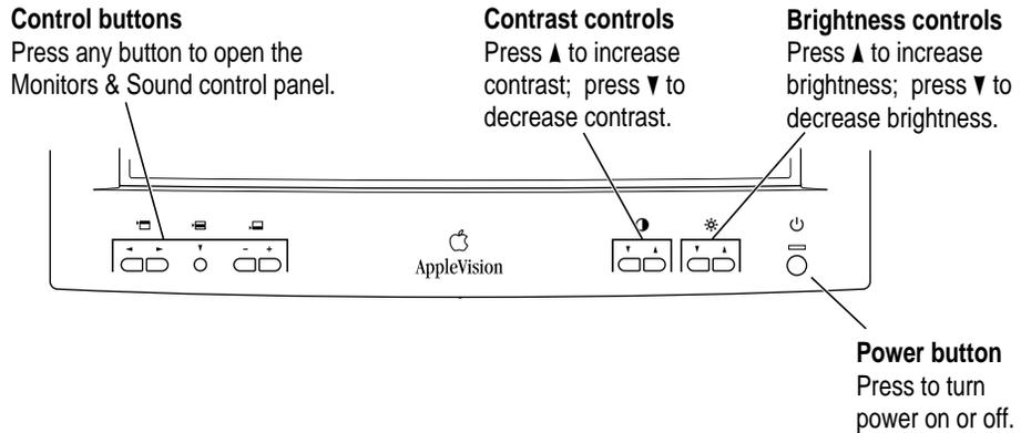
The Contrast and Brightness adjustments have an onscreen indicator that appears when you press a button on the front of your monitor. For example, pressing a Brightness button displays the Brightness indicator.
