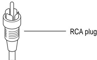
If your video equipment has an RCA-type plug and you don't have a composite video port on your Mac OS–based computer, you'll need an adapter to connect your video equipment to the S-video port on your computer. The adapter converts an RCA plug into an S-video plug. You can purchase one from an Apple-authorized dealer or electronics supply store.
