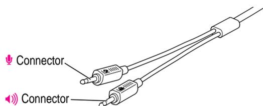
For Mac OS–based computers, the port (marked by 🎤) is on the back of the computer. For Windows-based computers, the connector (marked by 🎤) fits most standard microphone jacks. The sound input port on a Windows-based computer may be located on a sound or multimedia card.
