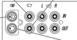
The S-video connector is a round plug with several small metal pins. You can plug the S-video input connector into your computer's S-video input port and the S-video output connector into your computer's S-video output port.
