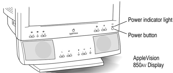
If you plug your monitor directly into your computer, no power indicator light goes on until you start up your computer. If you plug your monitor into a wall outlet, the monitor's amber power indicator light goes on. When you start up your computer, the indicator light turns green.
