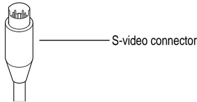
**IMPORTANT** The S-video connector resembles other Mac OS–based computer connectors, such as those for a printer, modem, mouse, or keyboard. Don't confuse the connectors; they are not interchangeable.
