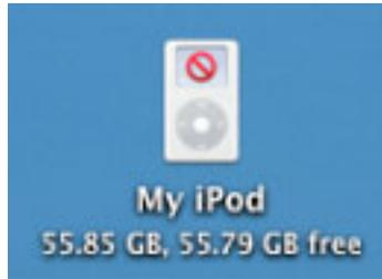
5. Drag a test file (40 MB or more) to the iPod desktop icon. If the file copies to the iPod without error, drag the iPod icon to the trash to eject the iPod. Fail the iPod if it does not function as expected.
