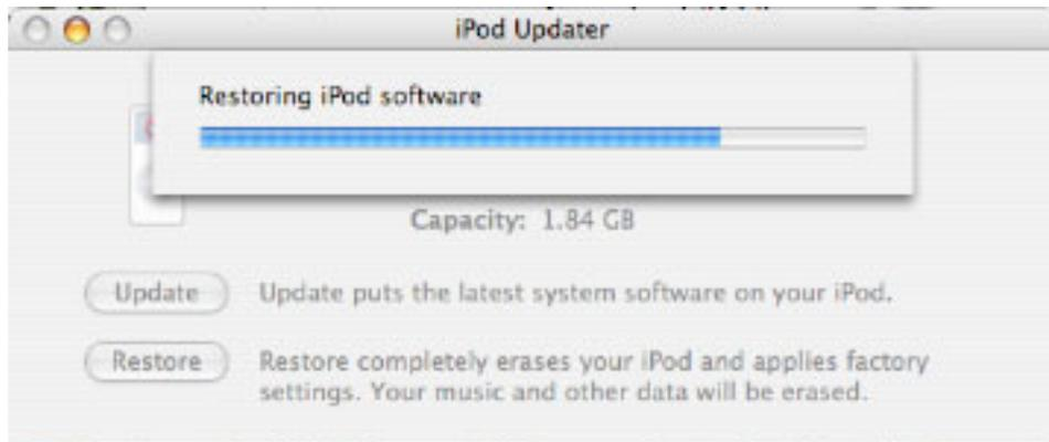
8. When the progress bar completes, in a few moments the message “Your iPod has been restored..., and is restarting.” appears on the computer.
