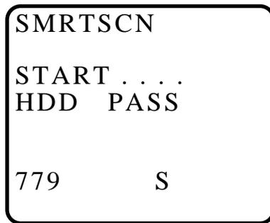
5. Pass condition = HDD PASS.
