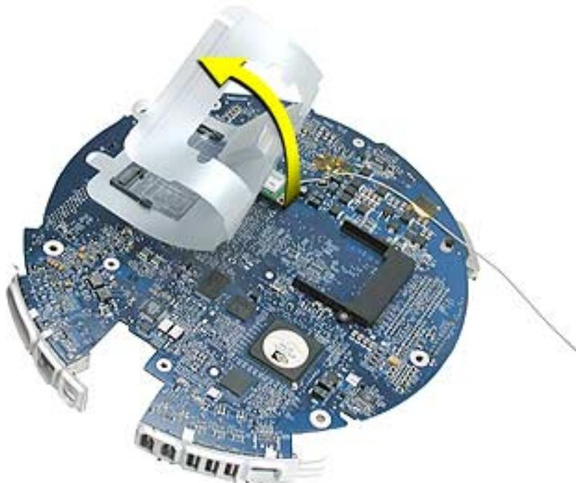
3. Remove the two screws (circled below) on the Bluetooth board. Peel back the Kapton tape to release the Bluetooth antenna. **Note:** You don't have to disconnect the Bluetooth antenna (shown by the arrow) from the board.
