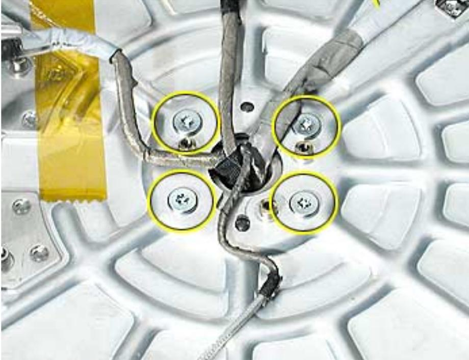
4. While holding the display bezel in this position, tighten the same four screws that hold the panel shield to the neck assembly.
