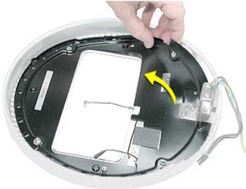
2. Remove two screws and lift the AC line filter from the bottom housing. **Note:** The port plug may fall out of the AC filter port when you remove the AC line filter. Replace the plug into the opening on the bottom housing before reinstalling the AC line filter.
