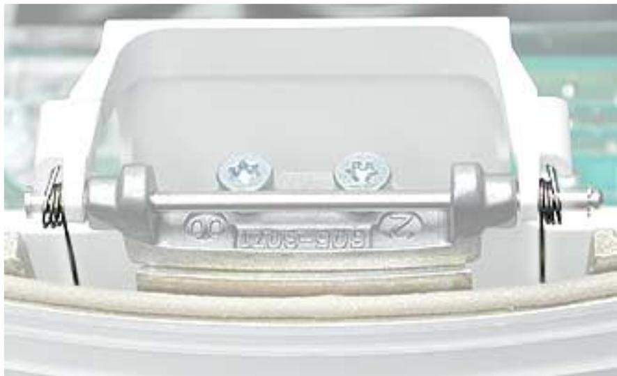
4. Remove the door hinge screws.
