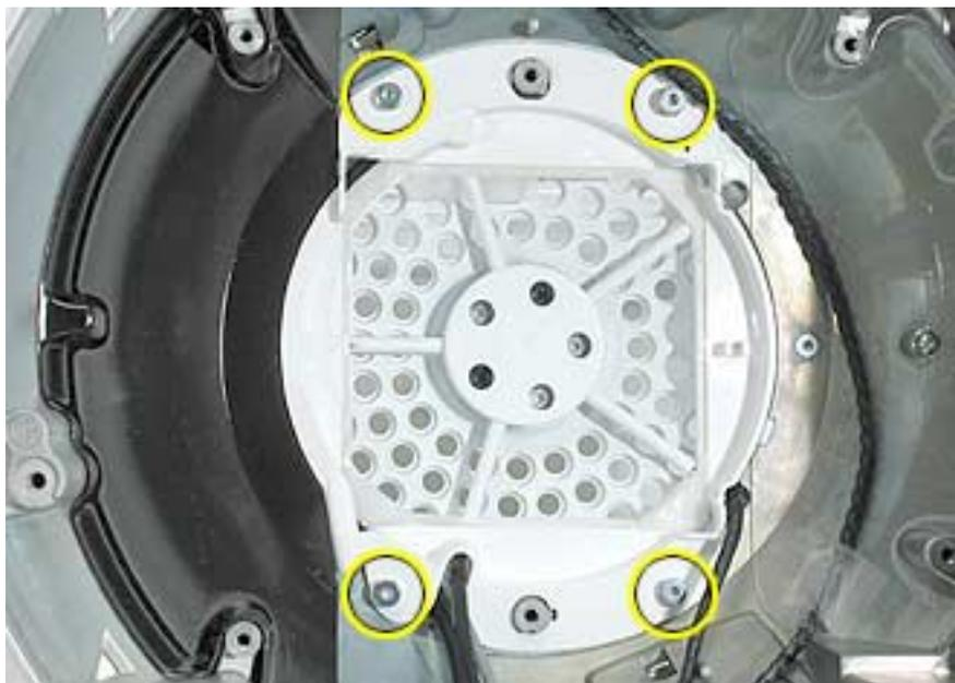
2. Lift the fan bracket out of the chassis. Note the orientation of the neck cables (see below) in the fan bracket before removing the cables. For orientation purposes, the drive door would be on the right.
