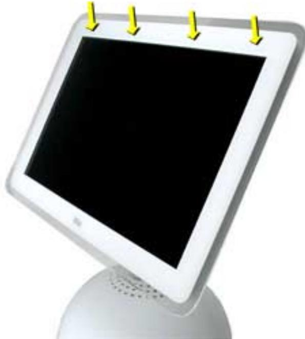
2. Holding onto the display, turn it over and lay the display face down on a soft cloth. Push the rear housing in the direction of the arrows. This will mate the housing and display tabs.
