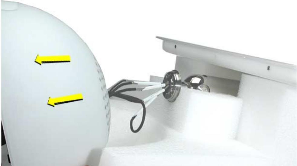
4. Remove one screw in the base of the Faraday cage to separate the white outer shell from the Faraday cage.
