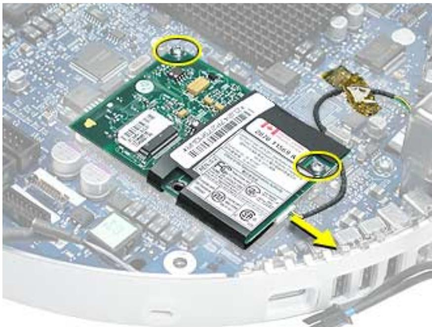
2. Lift the modem board from the connector on the logic board.
