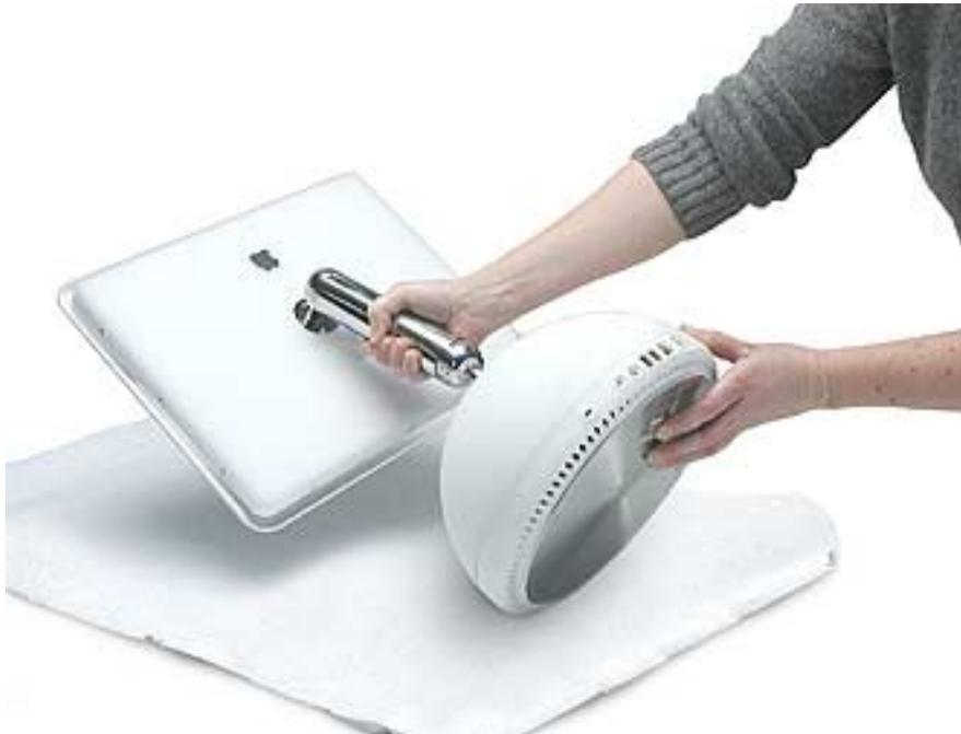
3. Loosen the four captive screws at the base of the computer and gently remove the access panel.
