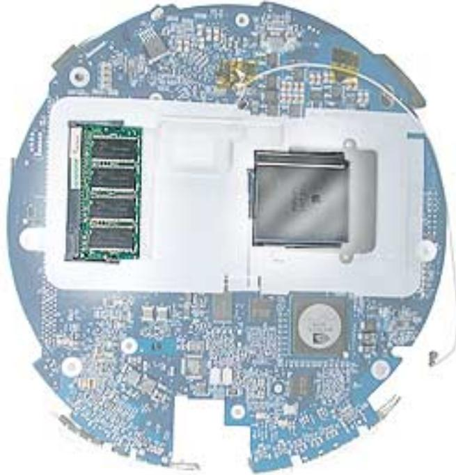
2. Remove the logic board protective cover to access the Bluetooth board
