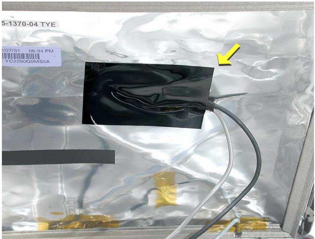
5. Disconnect the TMDS connector by squeezing the clip (1) on each side of the connector. Gently pull the cable (2) out of the slot.
