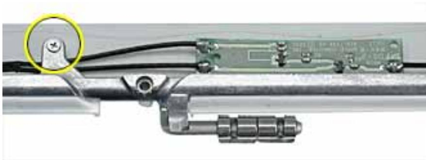
5. Lift up the bezel brace and release the cables from under the brace.
