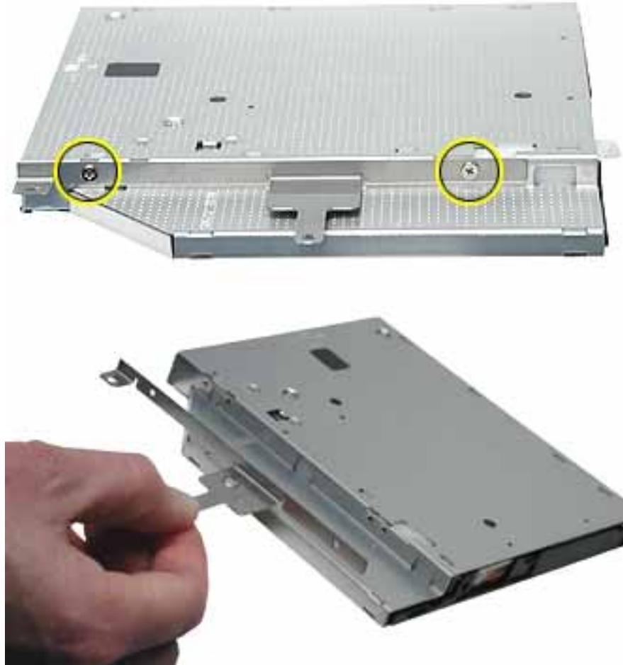
14. Install the replacement optical drive, and reassemble and test the computer.
