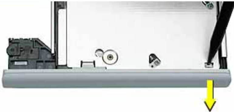
5. Press the wider tab, and pull the bezel off of the drive.
