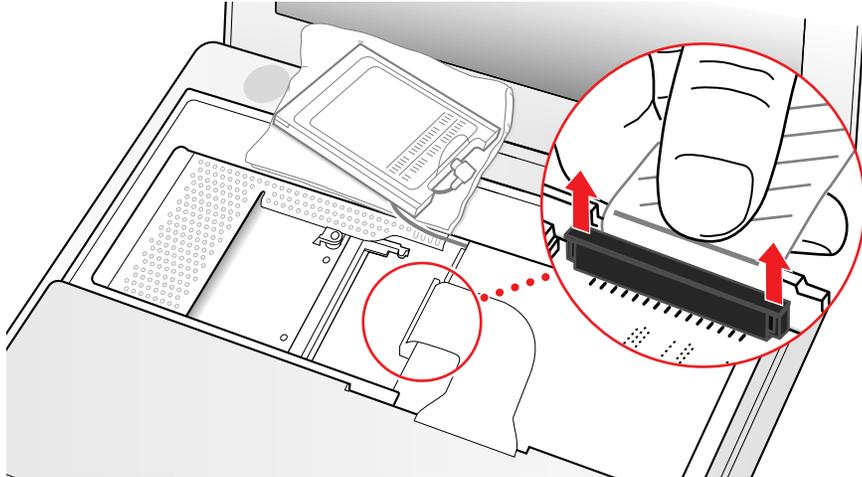
14. Install the replacement keyboard, RAM shield, and AirPort Card (if used).
