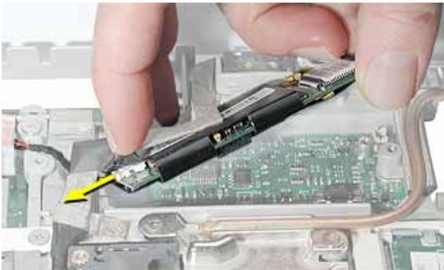
7. Install the replacement modem, and reassemble and test the computer.
