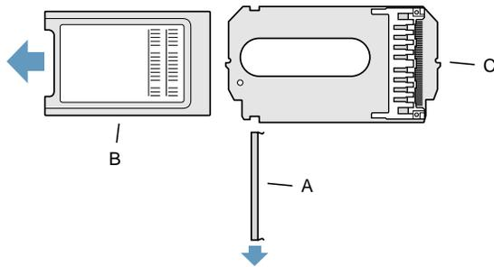
Plug the AirPort antenna cable connector into the port (located just below the pull-tab) on the end of the AirPort Card. Make sure the connector is straight before inserting it into the card.
