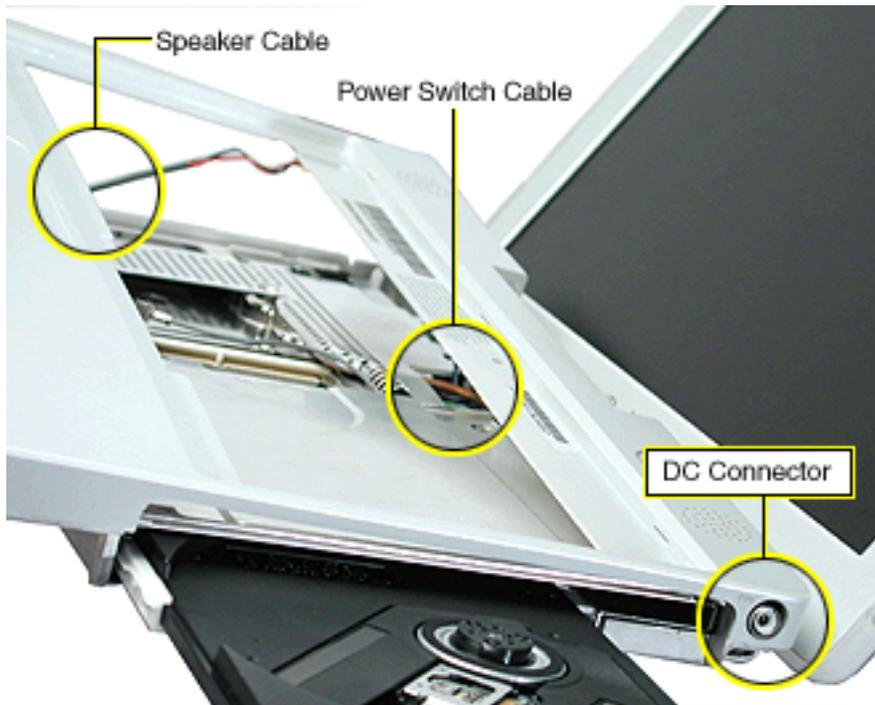
6. With the top case loosened, disconnect the speaker cable from the logic board.
