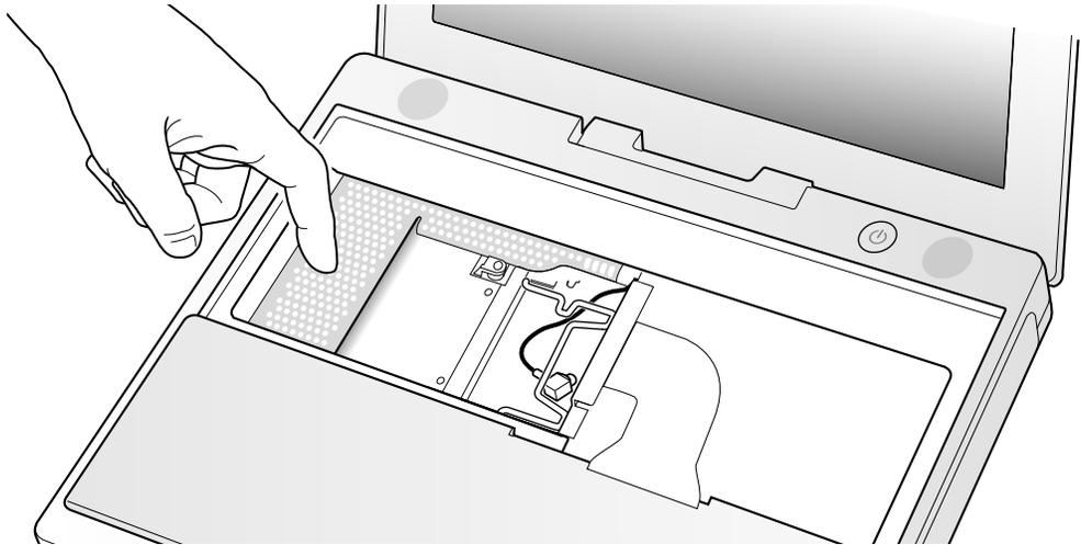
6. If the computer has the optional AirPort Card installed, unlatch the flexible wire holder that secures the card.
