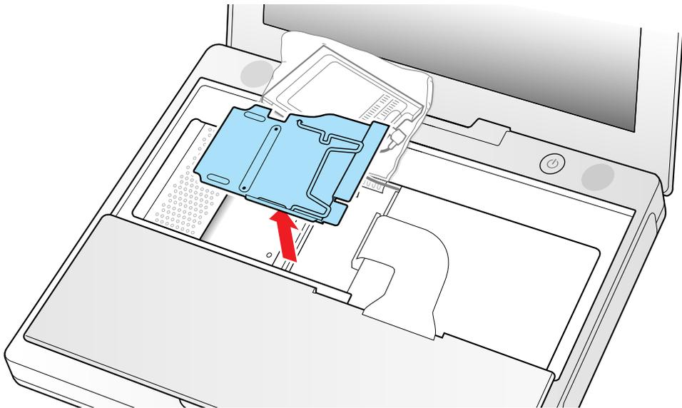
11. Locate the keyboard cable connector.
