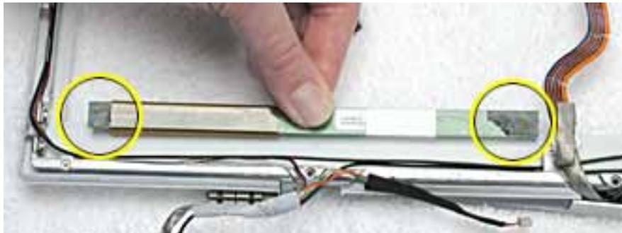
3. Install the replacement inverter board, and reassemble and test the computer.
