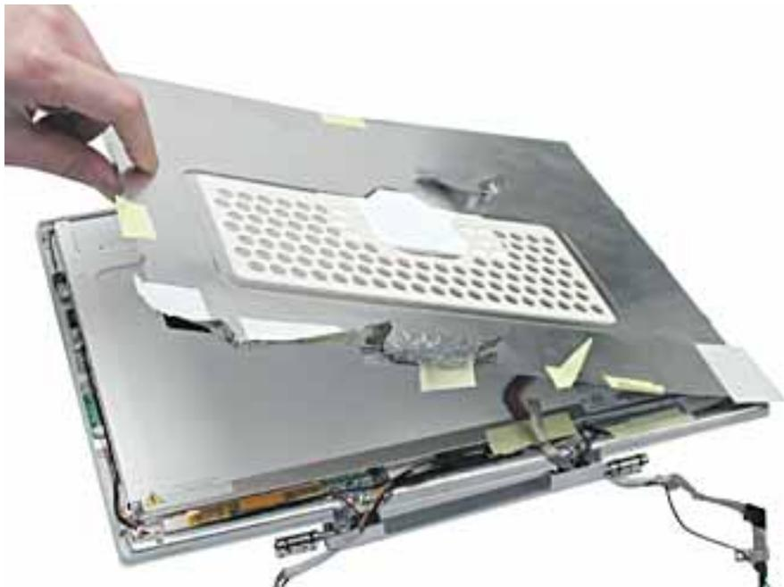
11. On the back of the LCD panel, grasp both sides of the LCD connector, and gently rock and pull the connector to disconnect the LCD cable from the LCD panel.
