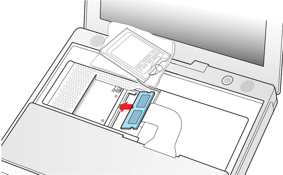
4. Gently push the top of the card down until the brackets snap onto both sides of the memory card to lock it into place.
