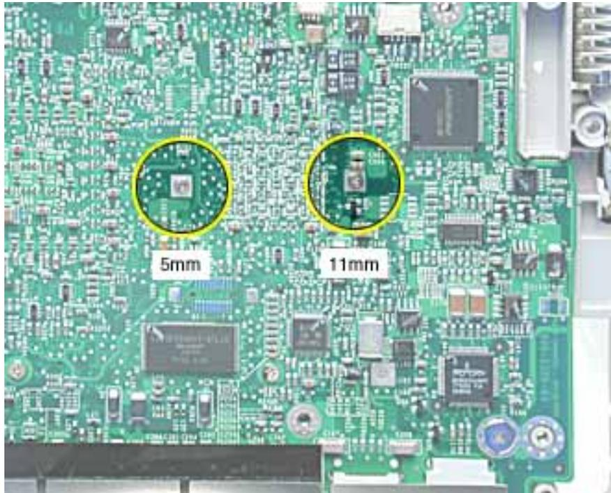
4. Remove the two screws holding the vent cover to the heat spreader.
