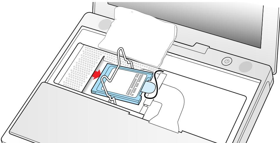
8. If an AirPort Card is not installed, unlatch the flexible wire holder to release the AirPort Card antenna cable.
