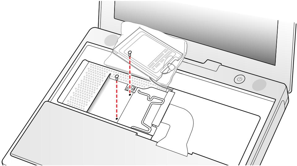
10. Lift the RAM shield out of the computer. Carefully pulling up on the wire holder may help to remove the shield.
