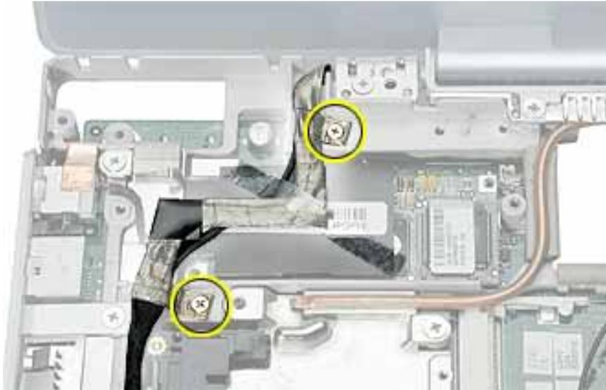
6. Peel the tape off of the computer frame, and disconnect the flat backlight cable from the logic board.
