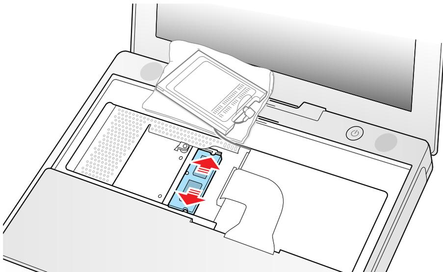
3. Install the replacement memory card by lining up the notch in the memory card with the small tab in the memory slot. Hold the card at a 30-degree angle, then push the card into the slot until it is firmly seated.
