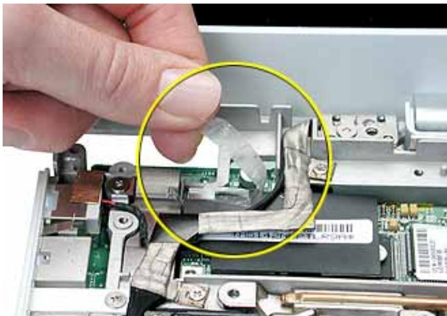
4. Tilt up the end of the modem board to disconnect it from the logic board.
