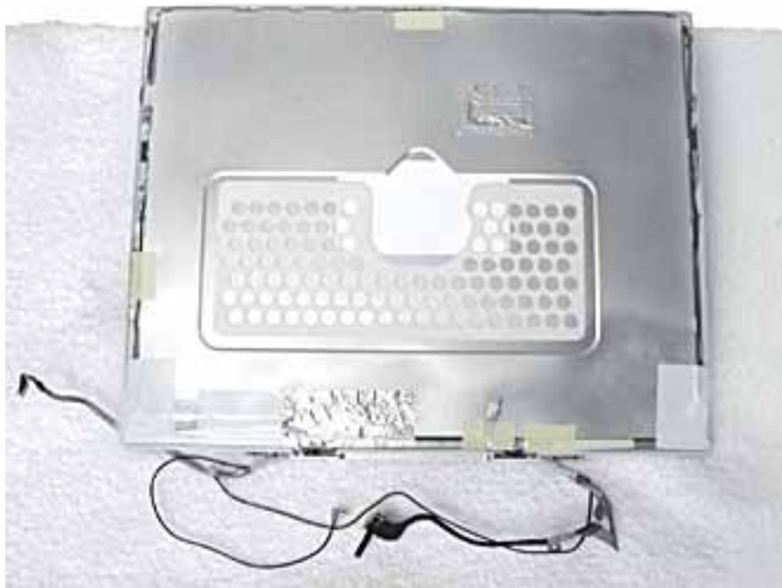
5. Peel up the tape if it covers the two screws at the clutch. Remove the two 11-mm long Phillips screws.
