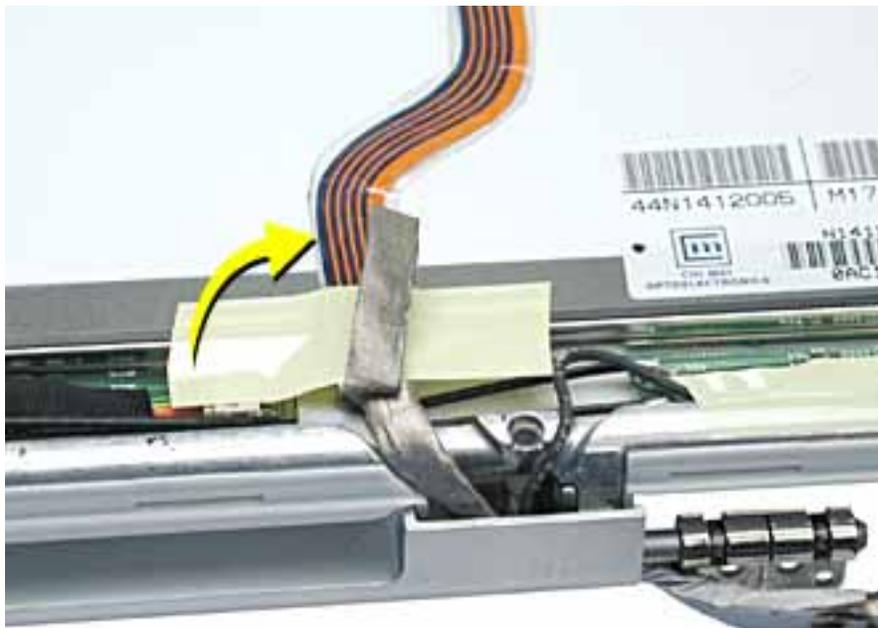
13. **Warning: When lifting the LCD panel, be careful not to strain the inverter cable.**
