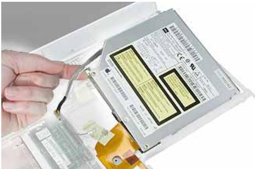
10. Remove the two screws holding the cable bracket to the optical drive.
