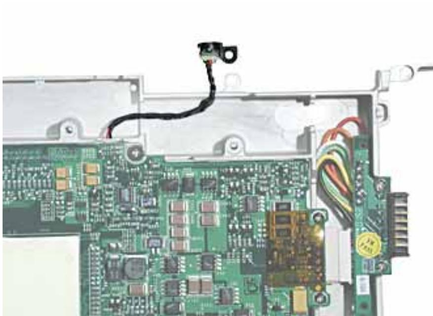
3. Turn over the computer frame and remove the two Phillips screws that secure the logic board to the heat spreader plate:
