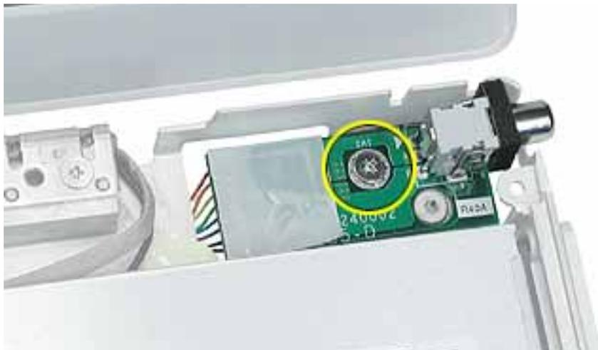
2. Tilt up the DC board and route it through the opening in the computer frame.
