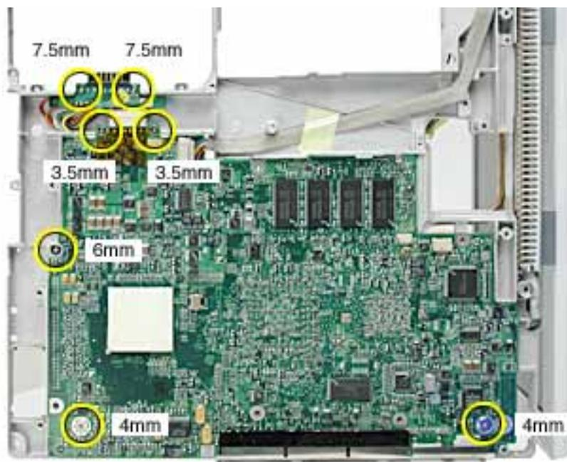
**Note:** When reassembling the computer, make sure that the underside of the replacement logic board includes the thermal transfer pad covering the large chip.
