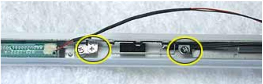
10. Tilt up the antenna receptor to remove it from the left side of the bezel assembly.
