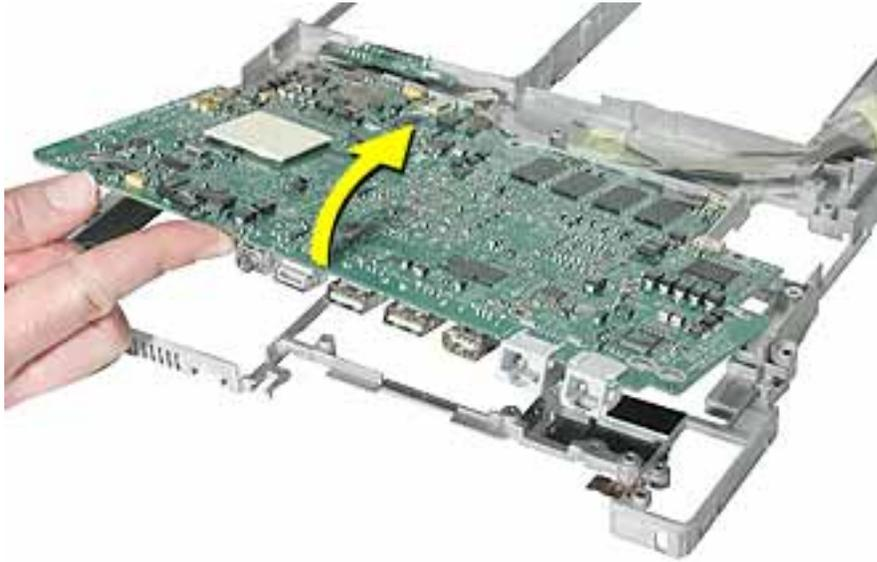
11. Disconnect the logic board from the battery transfer board connector.
