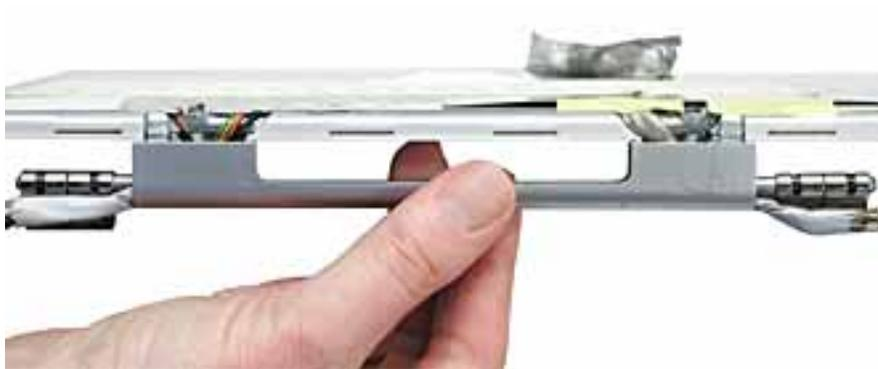
**Note:** The clutch caps are mirror images of each other. There is a right clutch cap and a left clutch cap. Note the positioning of the clutch caps on the display clutch cover. The image below shows the left clutch cap installed.
