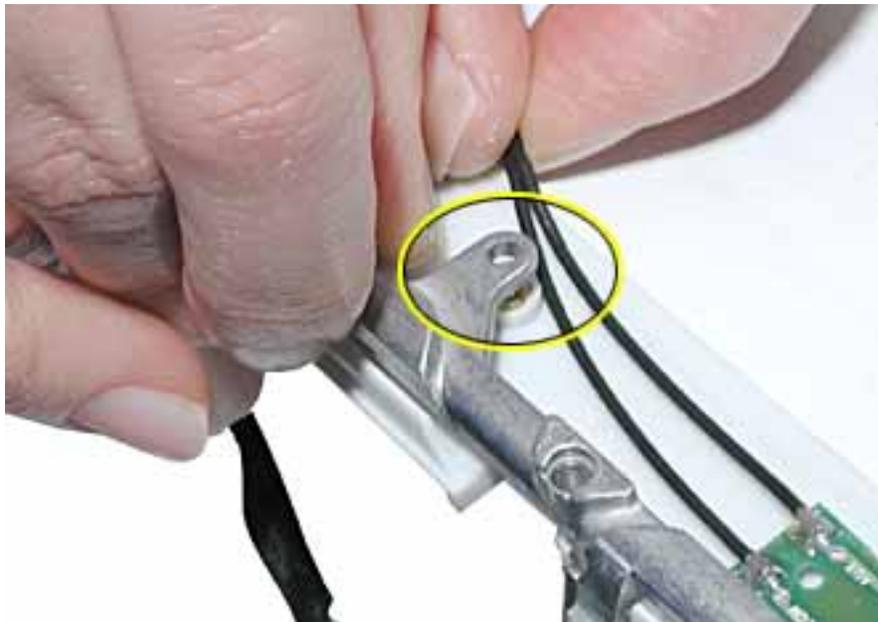
6. With the antenna board loosened, note the cable routing on each side of the bezel. On the right, the antenna receptor cable is routed underneath the microphone cable through two channels before terminating at the receptor bracket.
