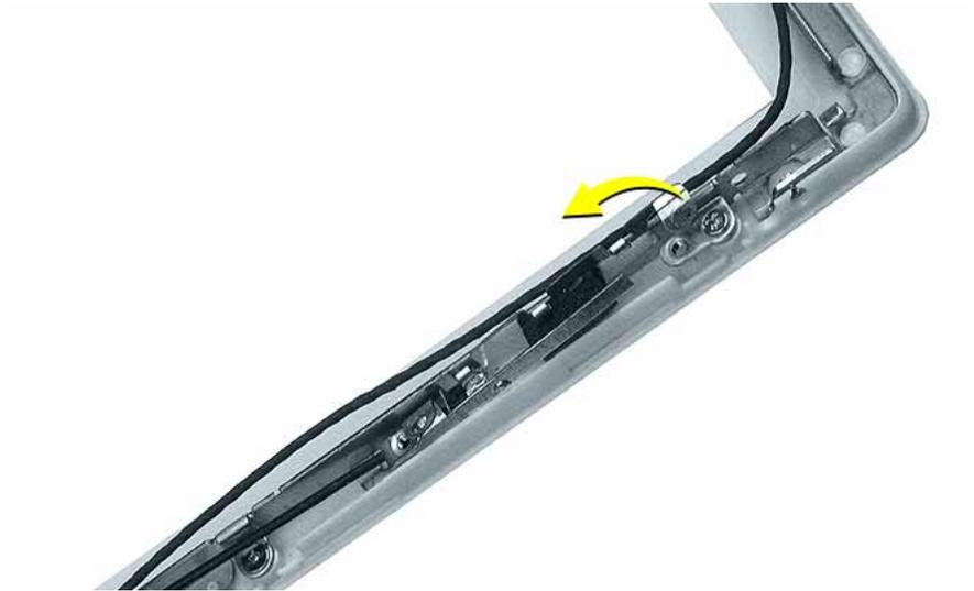
9. On the left side of the bezel, remove the two 3-mm long Phillips screws at the antenna receptor.
