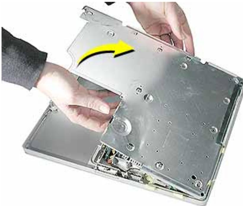
4. If necessary, use a black stick to separate the foil tape on the bottom shield from the I/O bezel shield.
