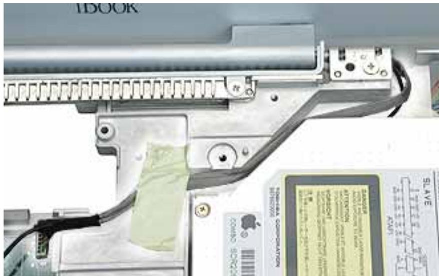
7. Route the cables up through the channel past the optical drive.
