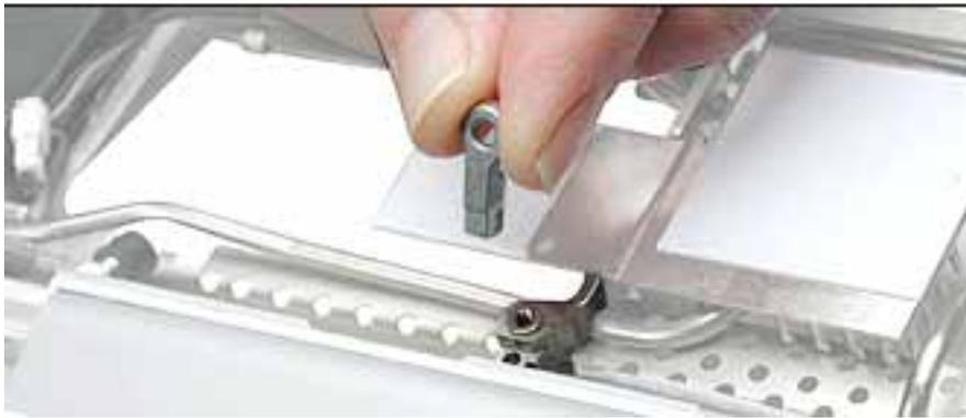
12. Remove the four identical black screws from the rib frame. (You might need to move aside the AirPort antenna cable to reach one of the screws.)
