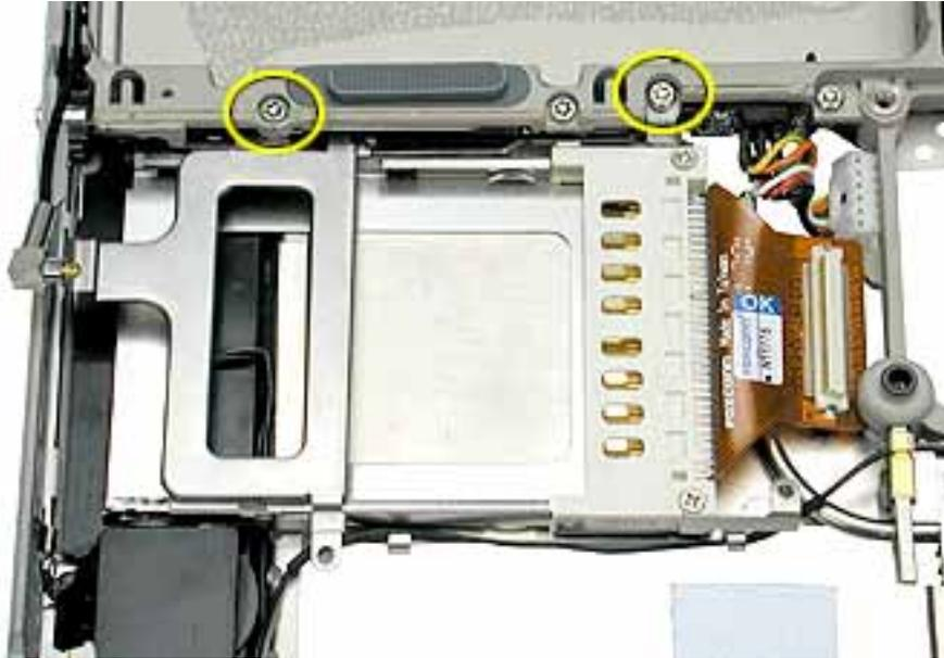
2. Lift out the PC card cage, being careful where it can catch on the PC card eject button.
