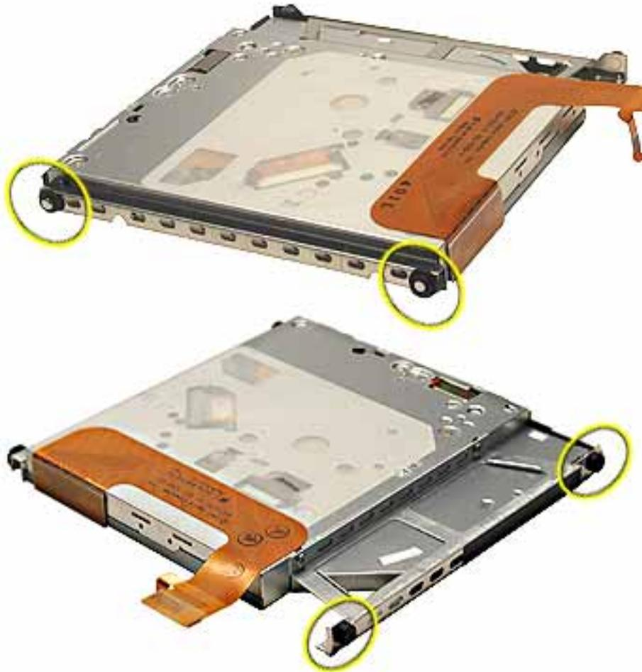
7. **Warning:** To prevent damage to the optical drive, handle the drive only by the corners. Do not press on the body of the drive.
