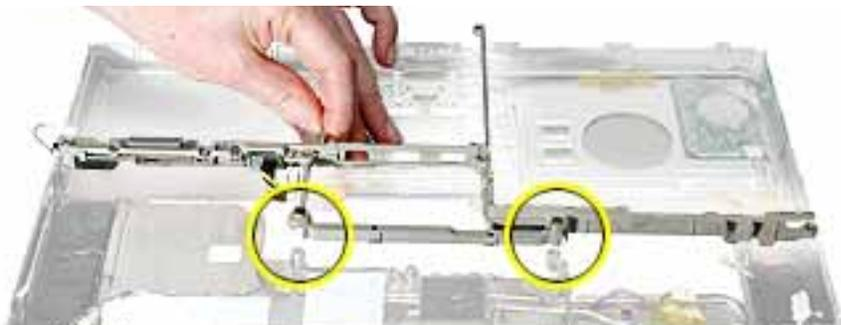
14. Disconnect the audio cable at each end of the heat exchanger.
