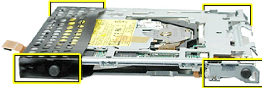
6. Gently pull up on the outer side of the drive to remove it.
