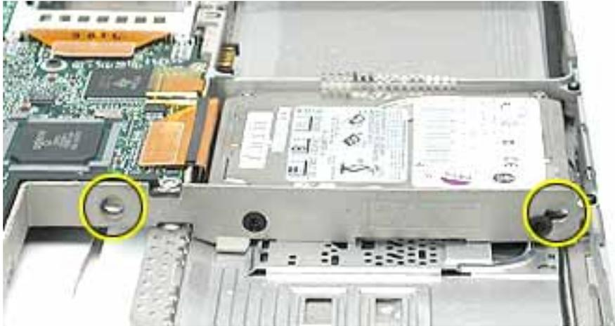
**Important:** When the rubber stoppers are inserted, push down on all four corners of the drive to verify that the drive is level and secure.
