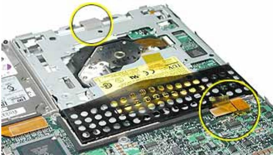
3. Locate the metal spacer that fits between the drive and the front bezel.
