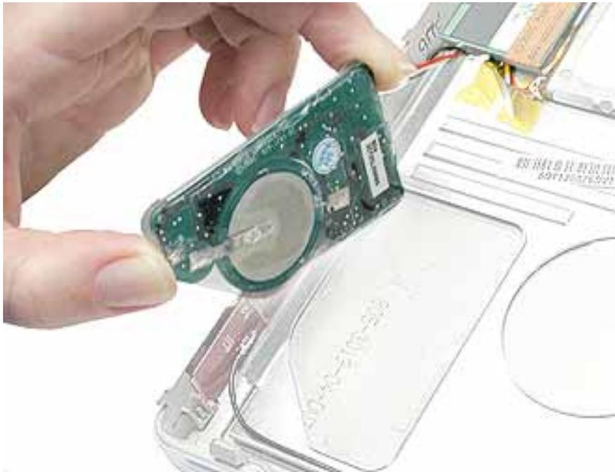
6. Install the replacement backup battery, and reassemble and test the computer.
