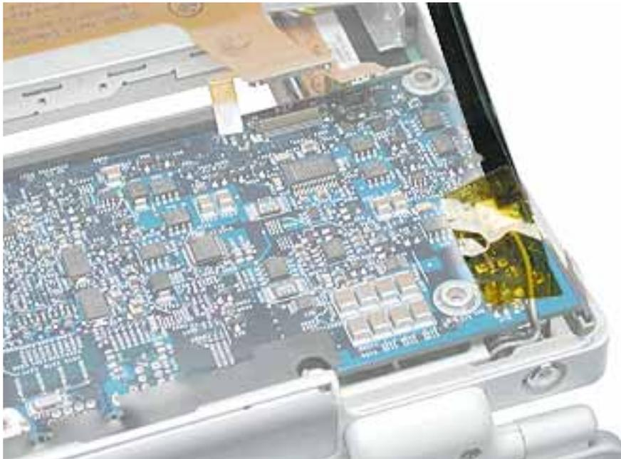
12. Grasp the logic board near the AirPort Card carrier. Gently tilt up the board, being careful where it catches on the back panel ports, integral mesh liner, and the disconnected cables.
