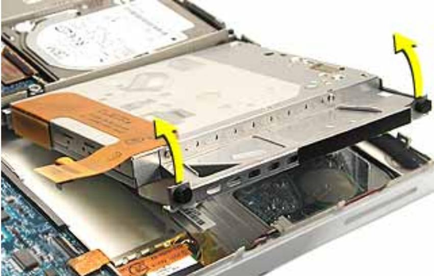
**Note:** There are four rubber stoppers (two on each side) on the drive that fit over metal posts at the corners of the drive. Remove any that may have fallen off inside the computer.
