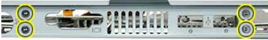
11. Lift out the two back panel mounts from the notches in the rib frame.
