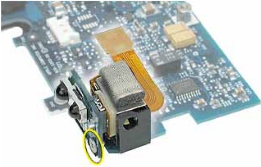
15. Remove the infrared communications board for installation on the replacement logic board.
