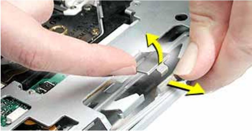
**Note:** When installing the replacement drive, insert the hooks on the metal spacer into the drive chassis, as shown.
