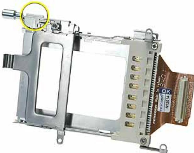
4. When installing the replacement PC card cage, ensure that the metal flange that is closest to the PC card eject button goes underneath the rib frame and metal liner at the battery latch.
