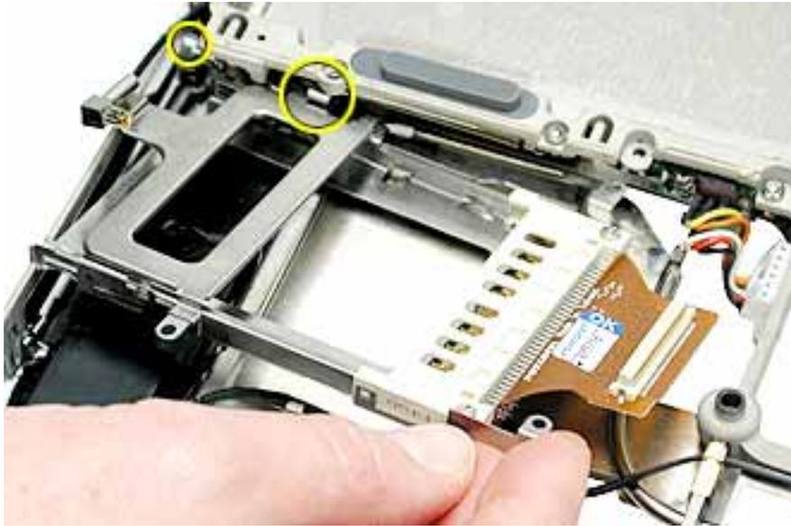
5. Install the replacement PC card cage, and reassemble and test the computer.
