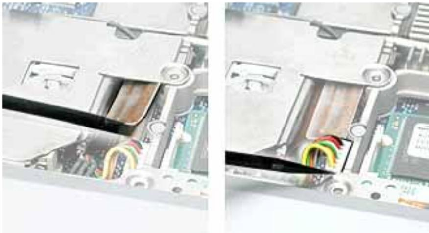
**Note:** When reassembling the computer, tuck down the battery cables so they do not get in the way when the keyboard is installed.
