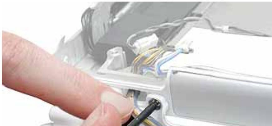
7. At the right clutch, note the routing of the inverter cable. Without straining the inverter cable, gently move it aside so you can access the two large silver-colored screws.
