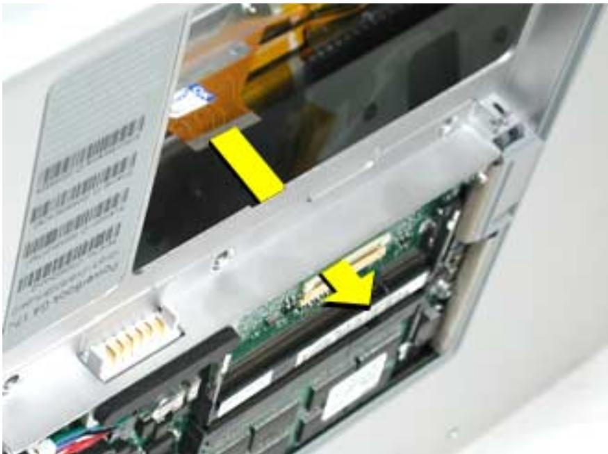
**Note:** For the following procedures, you will want to keep the top case close to the bottom case so the flex cable will not pull out of the slot.
