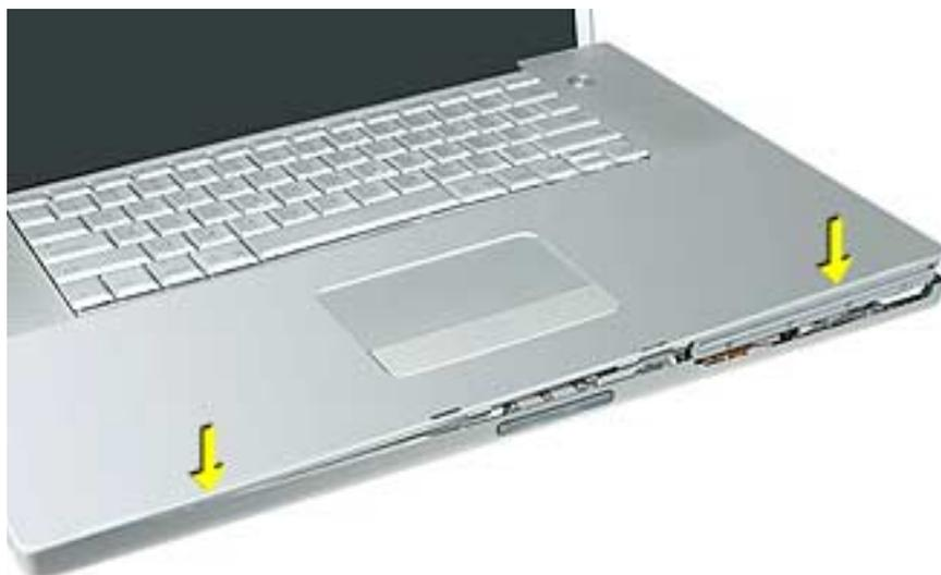
18. **Note:** If the tabs along the sides of the top case catch on the bottom case, use a narrow tool and work from front to back to carefully push or pull the tabs very slightly to help slide them into place.
