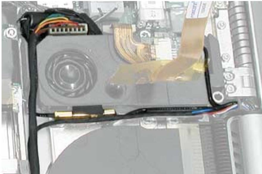
13. Verify that the LVDS cable's metal bead fits into the metal channel (rounded side up so that its teeth secure it) and that the cable is secured into the channel along the right speaker. Then, reconnect the LVDS cable and verify that it does not go over the fan.
