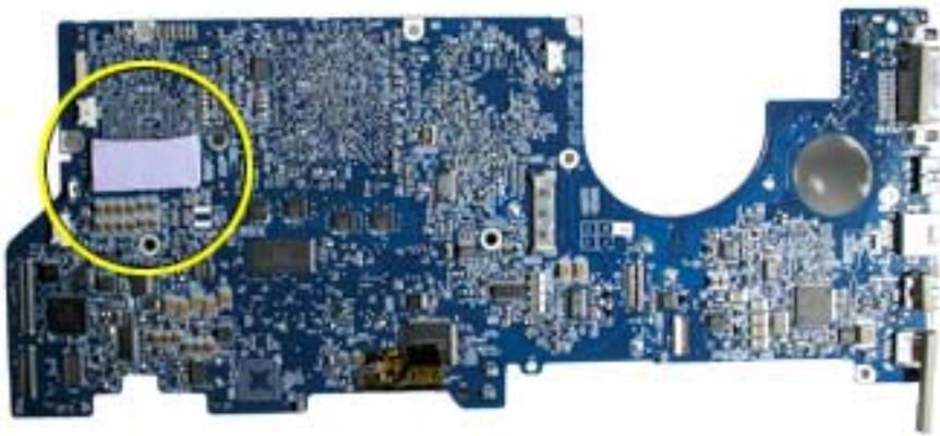
4. Use a black stick to remove all the original thermal material on the heatsink at the locations shown below.
