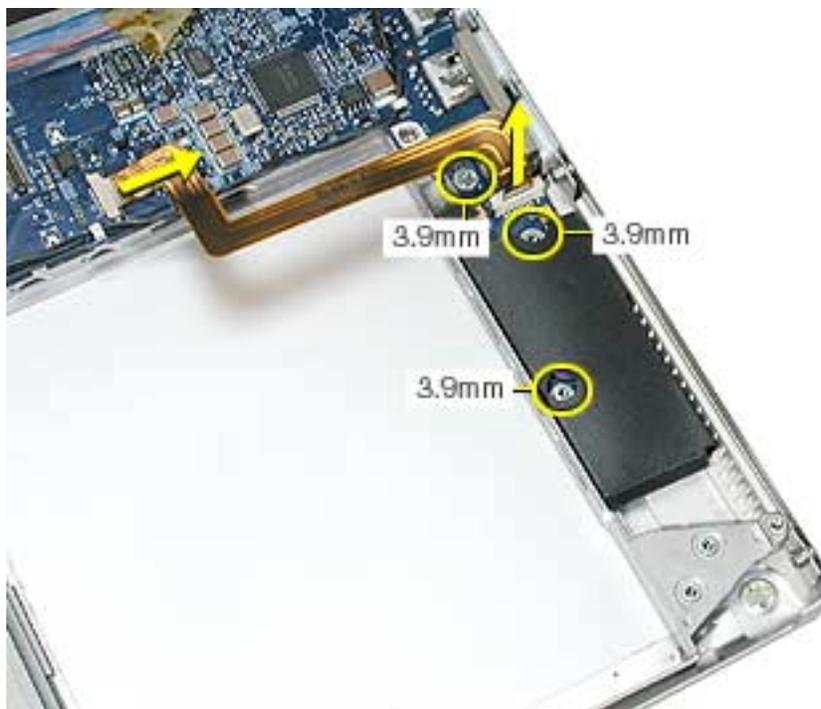
3. Install the replacement backup battery board.
