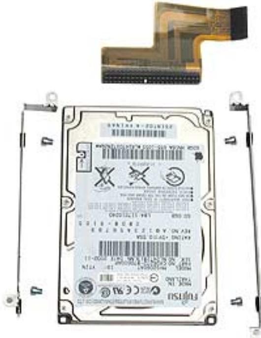
6. Install the replacement hard drive, and reassemble the computer.
