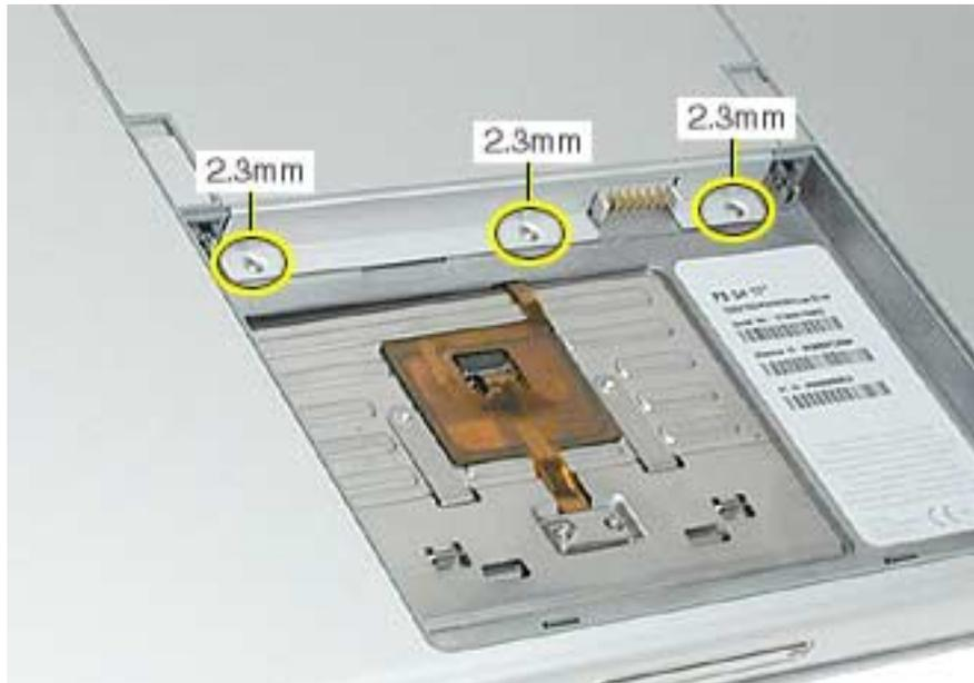
3. Lift the memory door up slightly and slide it straight back to remove.
