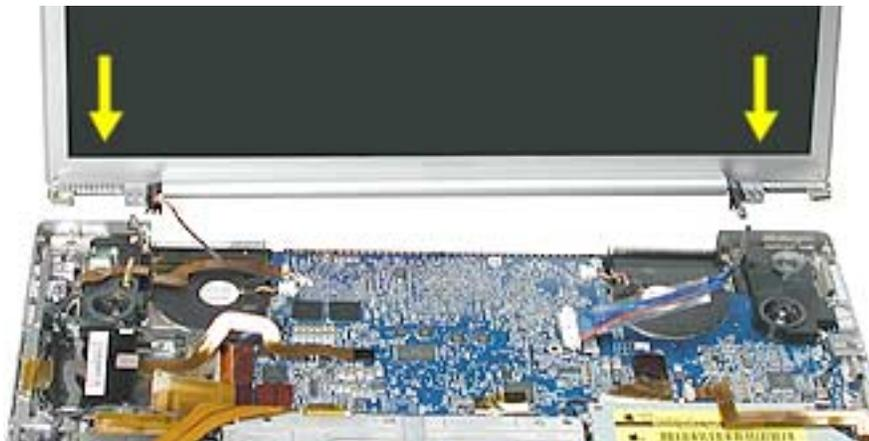
5. Verify that the limit stop feet, fit into the holes in front of the pop-up spring pins, on both sides.
