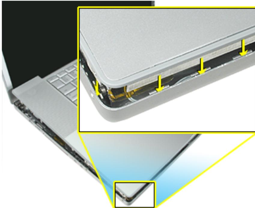
17. Hold the front of the top case along the front edge of the bottom case and lower into place.
