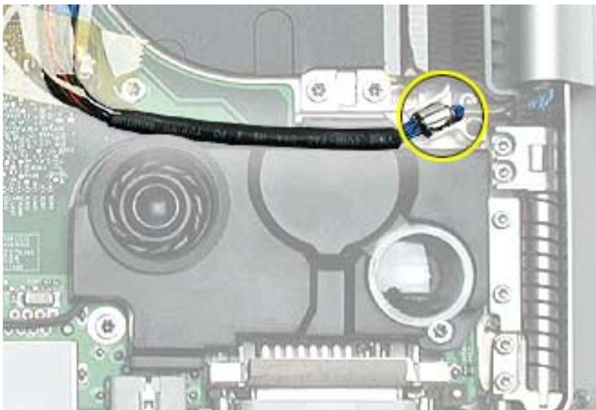
7. Verify that the sleep LED wires route over the notch in the frame (secure with Kapton tape) and along the inside channel away from the front edge so that it will not be damaged when replacing the top case.
