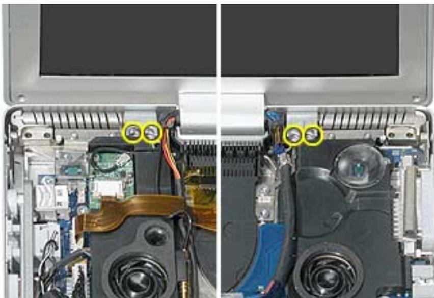
7. Lift off the display panel and clutch barrel assembly.
