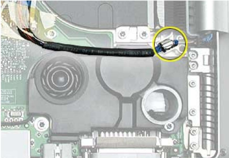
14. To verify that the pop-up mechanism was installed correctly, first make sure there are no wires or parts to interfere, then carefully close the display until it latches.
