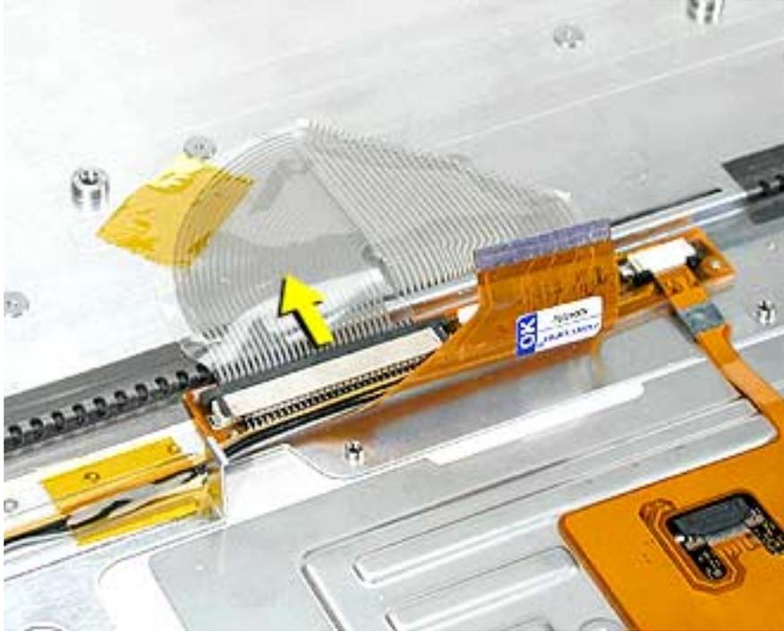
3. Locate and carefully peel off the insulator film over keyboard screws and reserve for reinstallation.
