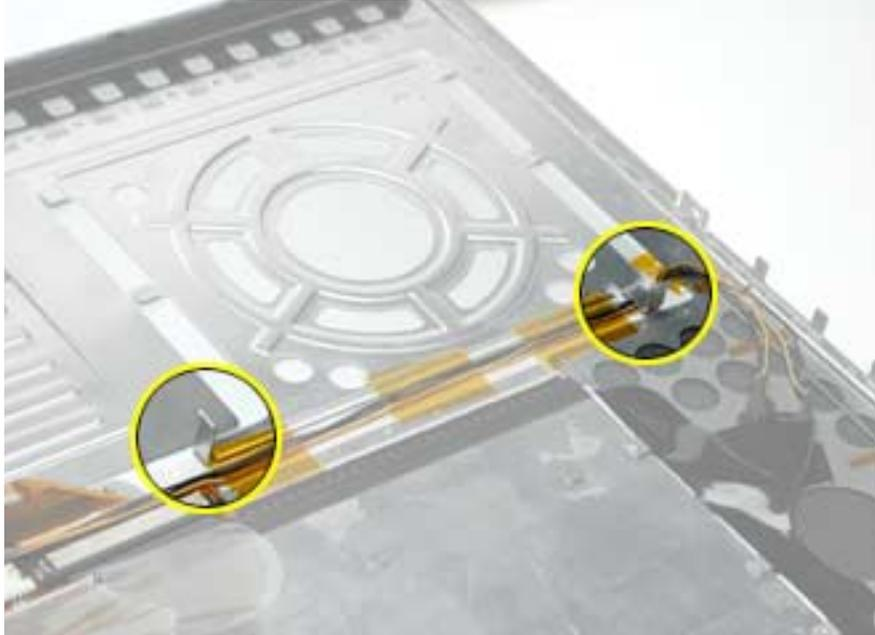
19. Install the front and rear side screws on both sides to hold the top case in place.
