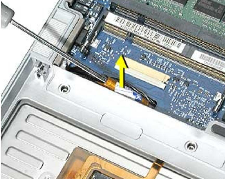
23. Carefully pull the locking bar of the ZIF connector out slightly. Slide the flex cable over the locking bar and into the connector until it stops (the metal edge of the cable should be parallel to the connector), then slide the locking bar in to secure it.
