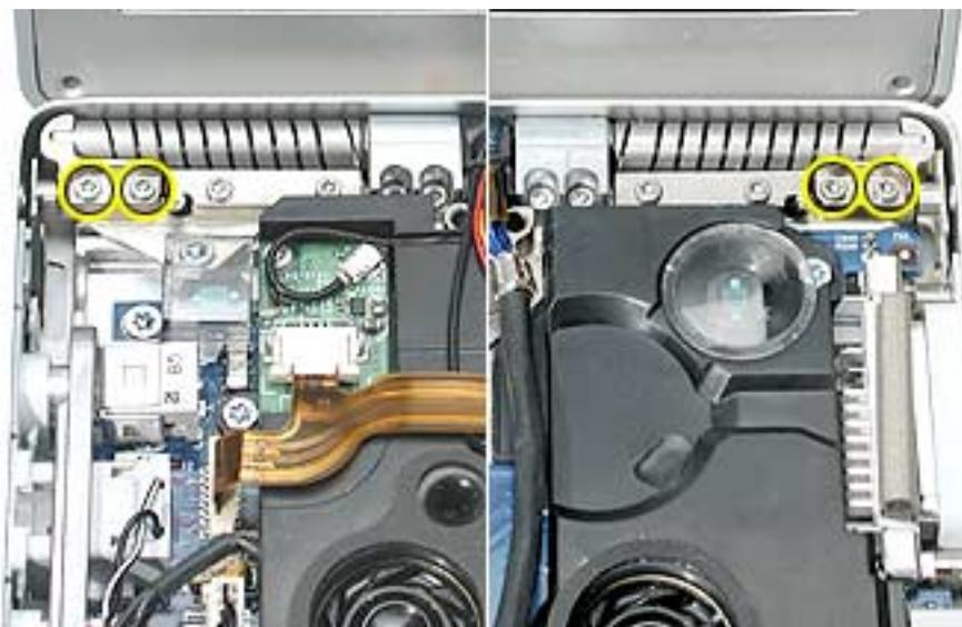
8. To install the pop-up torsion bars, insert the bar so that the notch is behind the pop-up spring pin and install the first screw furthest away from the pin.
