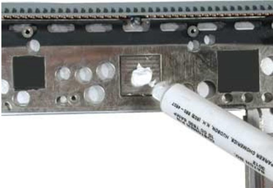
**Note:** After installing new thermal material, if you must briefly re-separate the logic board from the heatsink, it is OK to retain the same, new material, as long as they are not handled excessively.
