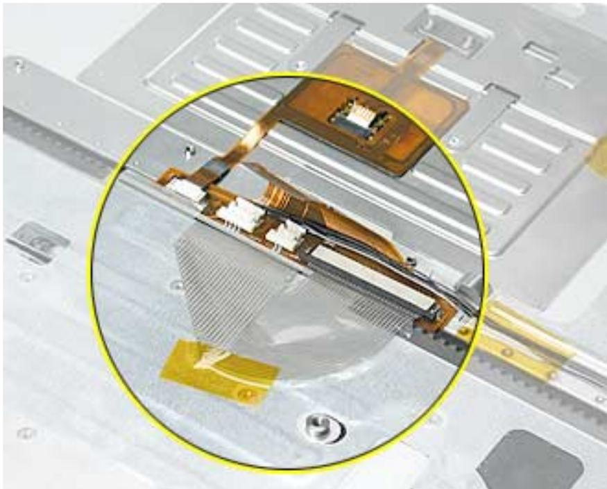
9. Verify that the cable is still fully inserted, straight and secure in the connector.
