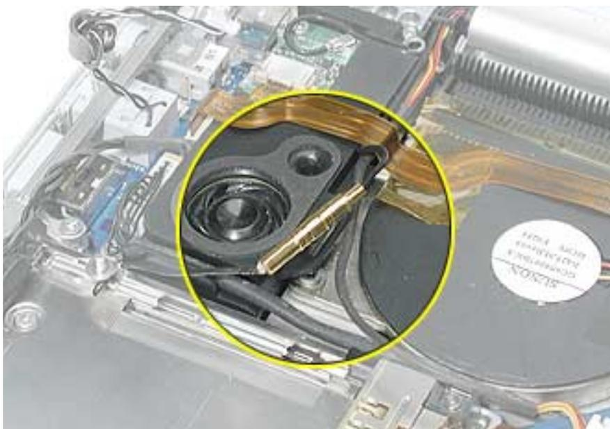
3. Carefully disconnect the Bluetooth cable connector.
