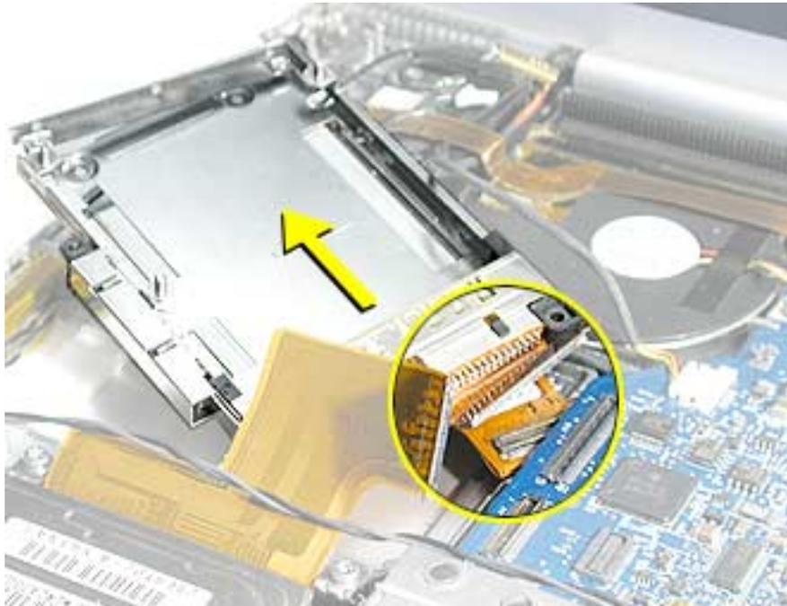
6. Slide out the PC card cage eject button.
