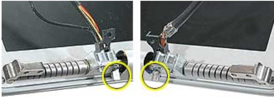
4. Lower the display panel assembly straight down onto the bottom case assembly.
