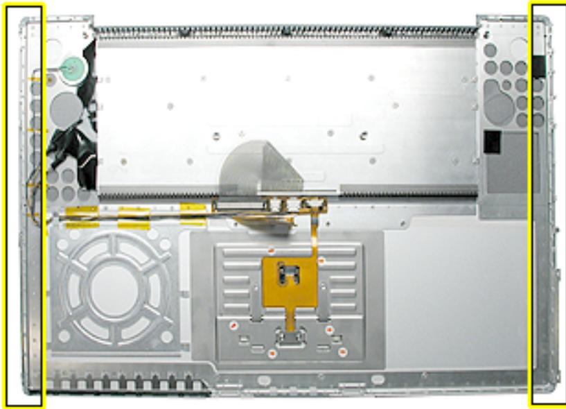
10. Lay the top case upside down and locate the flex cable.
