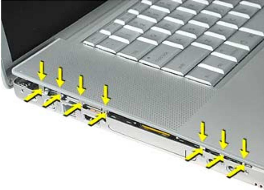
**Note:** Some side screws have a flexible screw boss. If they block a tab from seating, use a narrow tool to push the boss slightly.
