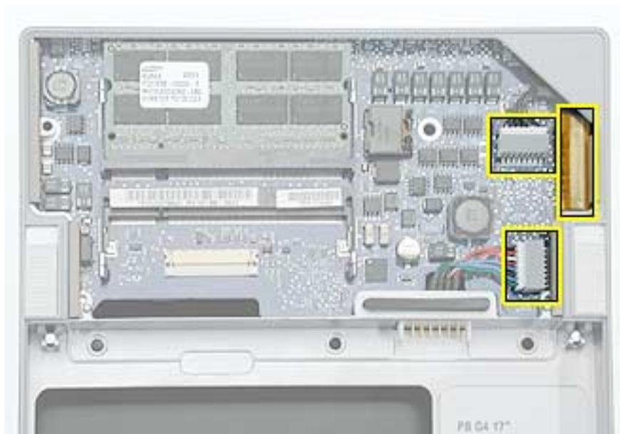
2. Turn the computer over. Disconnect the cables shown.
