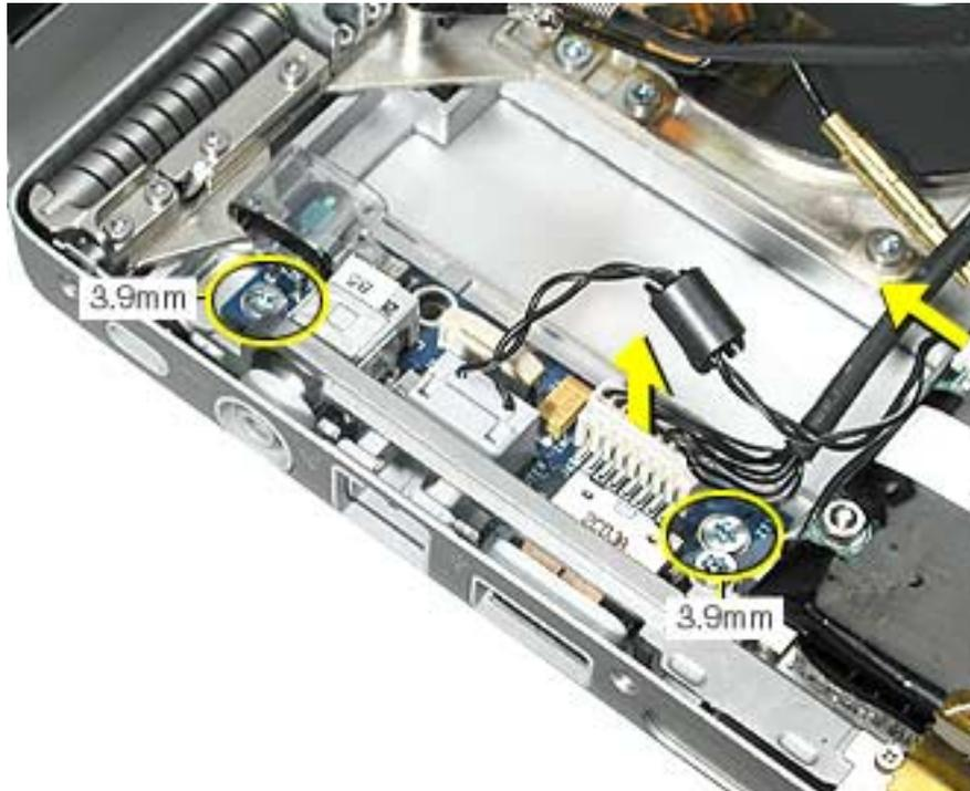
4. Insert a black stick under the DC-in board to help guide it out.
