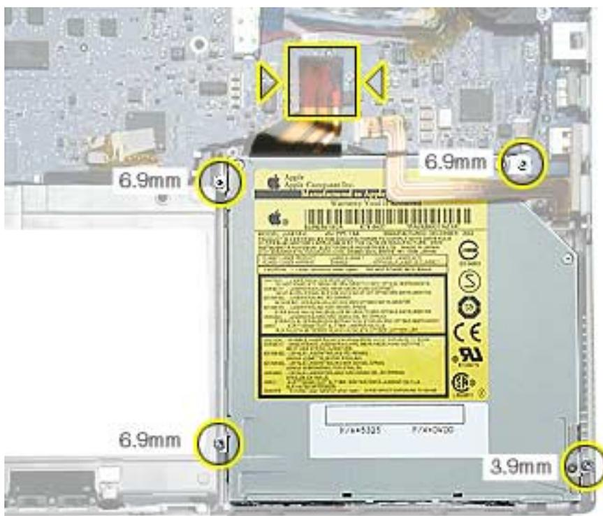
4. Transfer the flex cable, brackets and screws to the replacement SuperDrive.
