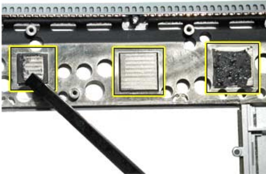
**Warning:** Whenever the logic board is separated from the heatsink, you must remove all existing thermal material and install new thermal material to the heatsink at the three locations shown above. Failure to do so can cause the computer to overheat and be damaged.
