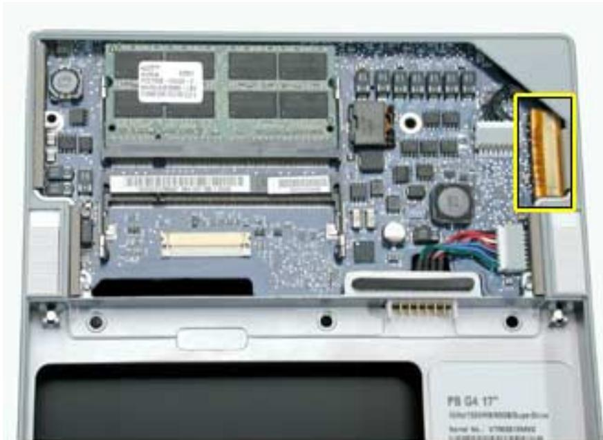
2. Turn the computer over and disconnect the PC card cage and hard drive flex cables.
