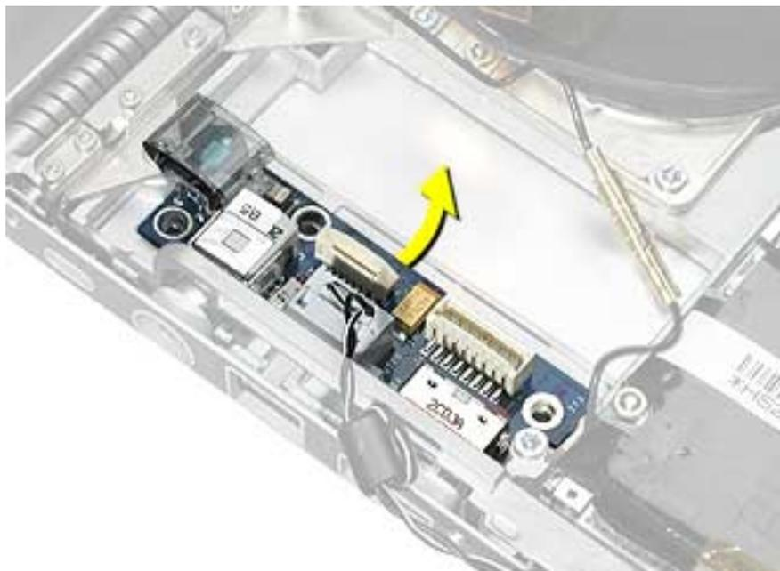
**Replacement Note:** Make sure that the replacement DC-in board includes the RJ-11 port and ambient light sensor cover. If not transfer them from the original board to the replacement board.
