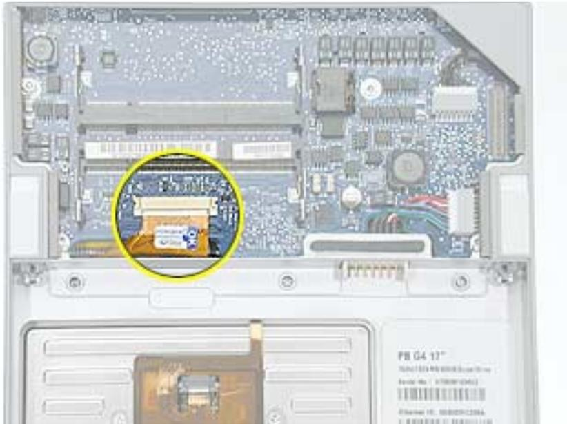
6. Very carefully disconnect and remove the cable from the connector.
