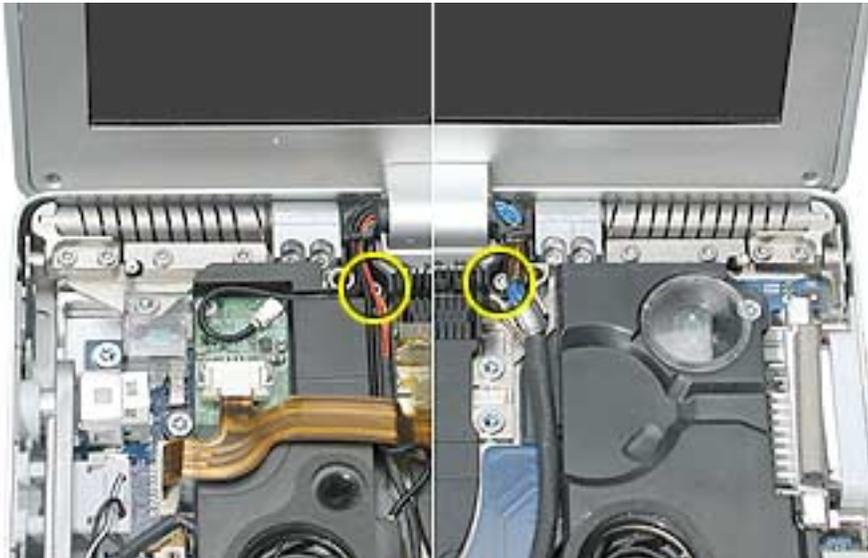
11. The left speaker has channels for Bluetooth, AirPort Extreme, inverter and the power cable from the DC-in board. Verify that the cables are routed and reconnected correctly.
