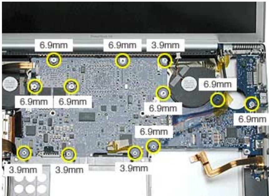
4. Lift the logic board from the left side and pivot along the port side.
