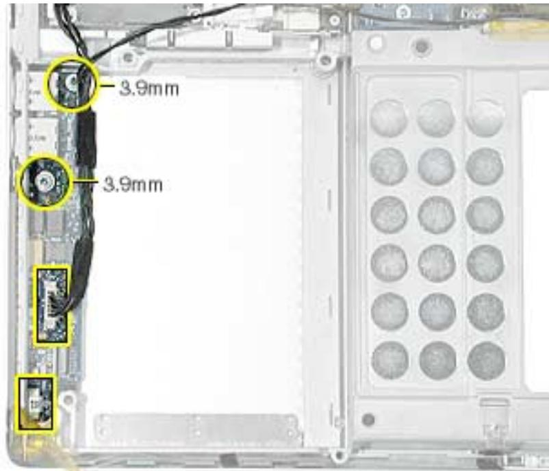
3. Pull the sound board out starting at the ports end.
