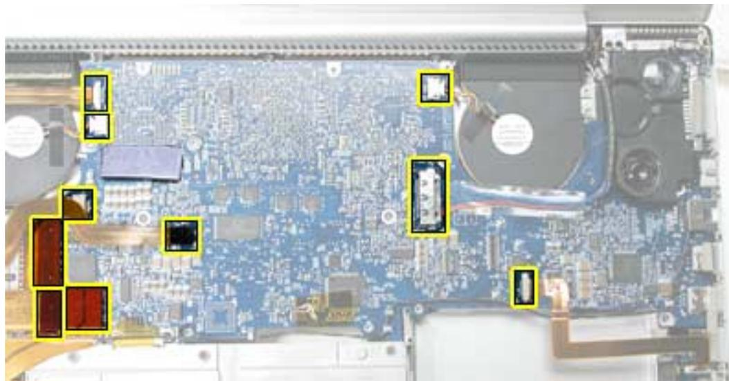
3. Check perimeter wiring, where shown, to verify that it will not be caught or pinched by the top case during replacement.
