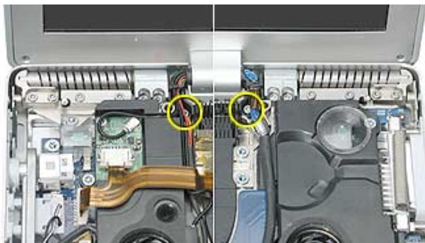
5. Verify that cables for Bluetooth, AirPort Extreme, inverter and power cable from the DC-in board are routed and seated correctly in channels around the left speaker.
