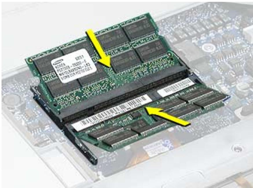
7. Check that the notches in the card clear the tabs as you press down on the sides of the card to lock it into place.
