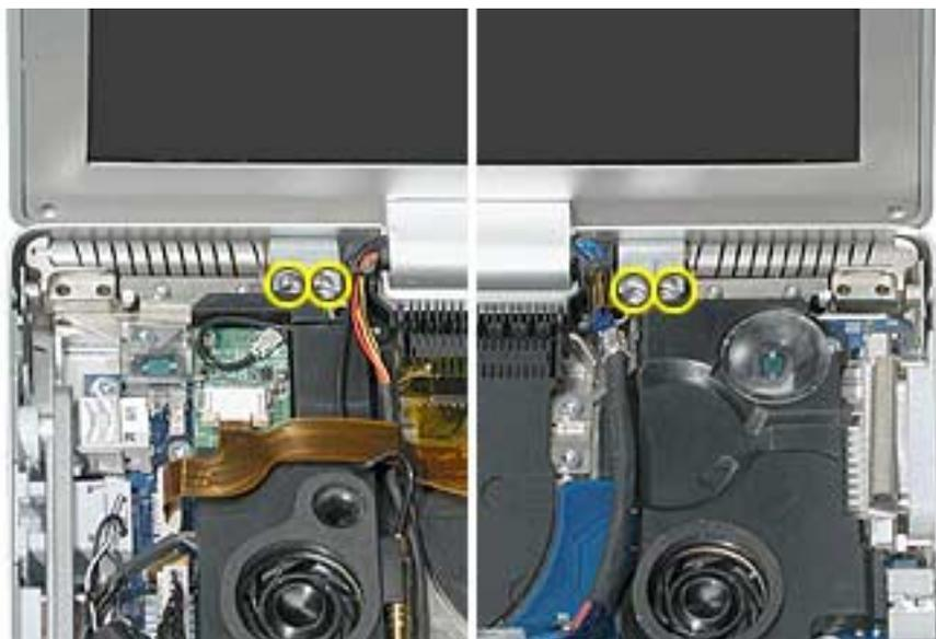
7. Hold the display at a 90-degree angle and install the end cap screws on both sides.
