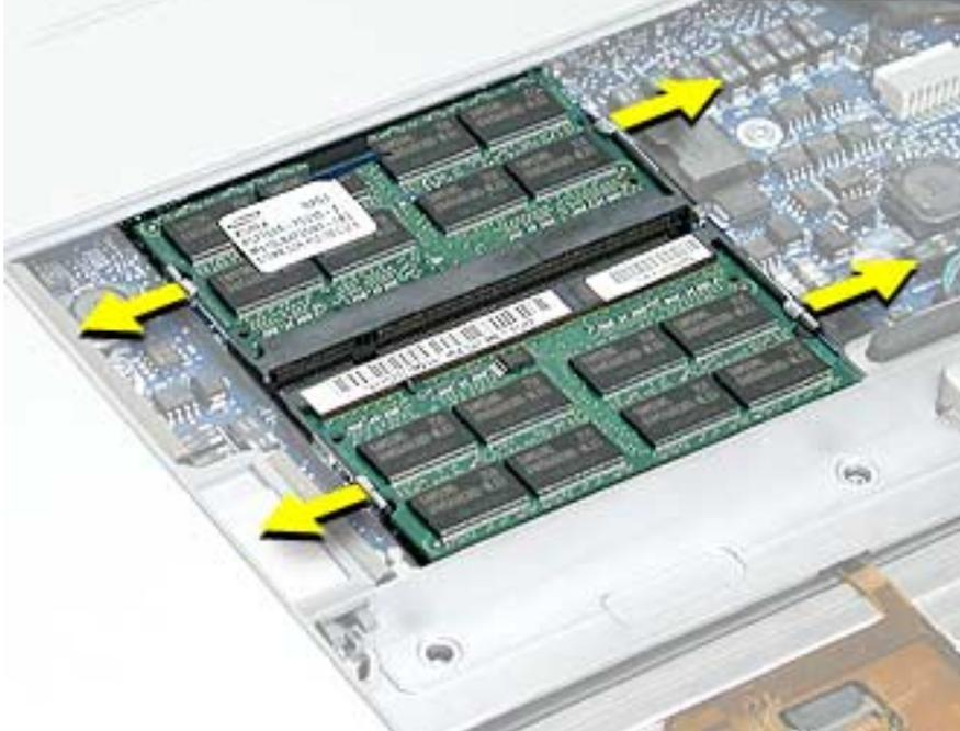
5. Pull the card straight out of the memory slot.
