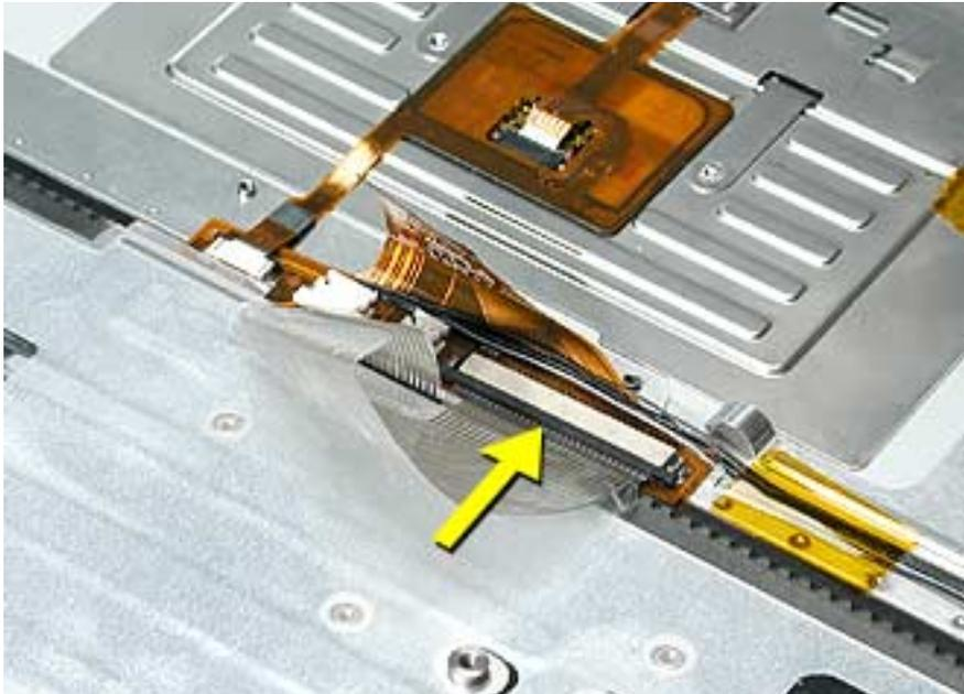
7. Fold the cable flat and secure its adhesive by firmly holding the left side (to prevent cable movement) while sliding your right hand fingers forward on the right side.
