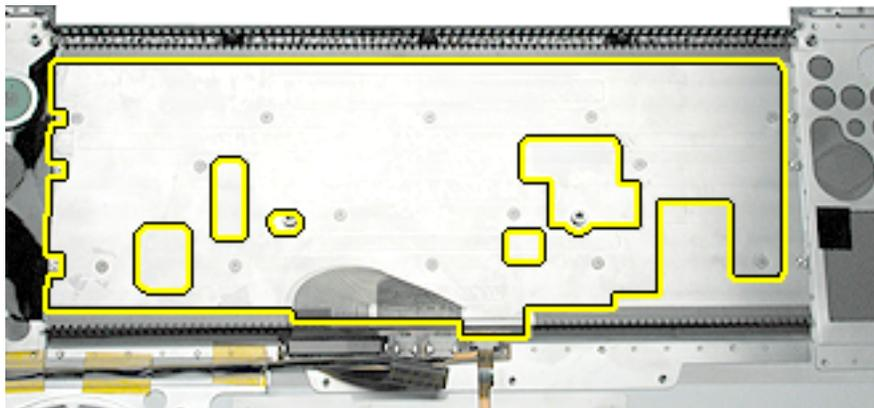
5. If replacing the existing keyboard, such as during a top case replacement, secure the end of the keyboard flex cable. (The cable inserts under the ZIF connector locking bar.)
