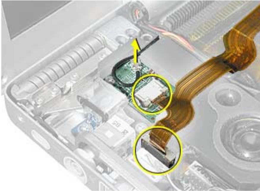
3. Remove the screw and Bluetooth board.
