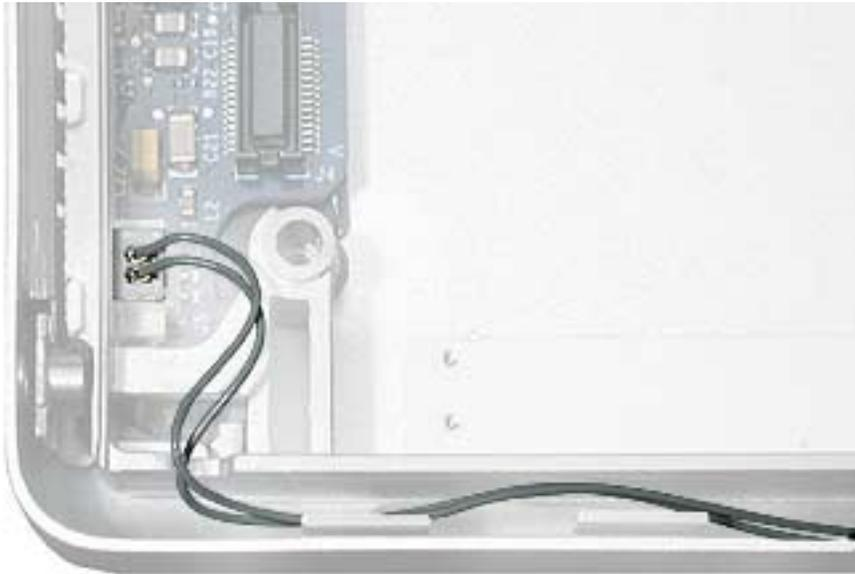
8. On the top case, check cable connections and routing.
