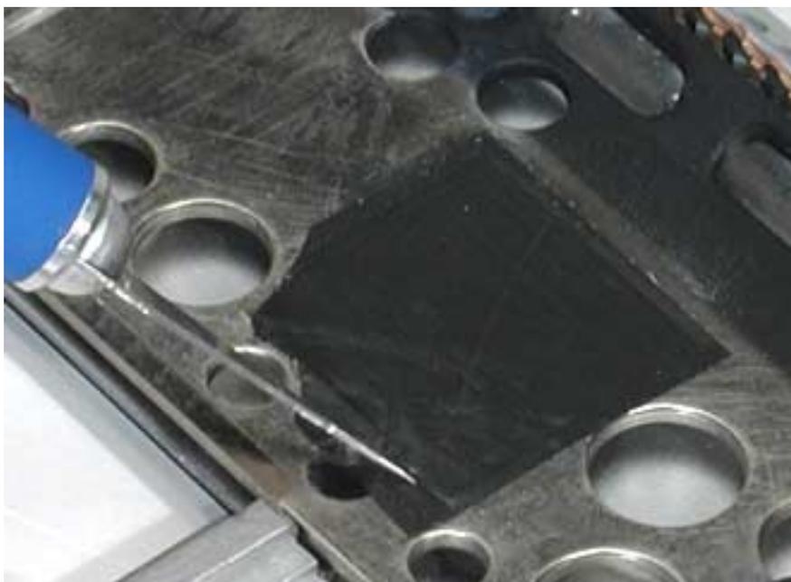
7. Apply approximately 0.3 to 0.5 cubic centimeter (cc) of T630 thermal gel (922-5929) to the center of the center mating surface on the heatsink. (The 10 cc dispenser may be graduated in milliliters. **Note:** A milliliter (ml) is the same as a cubic centimeter (cc)).
