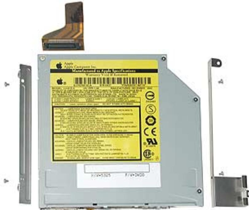
5. Install the replacement SuperDrive, and reassemble the computer.
