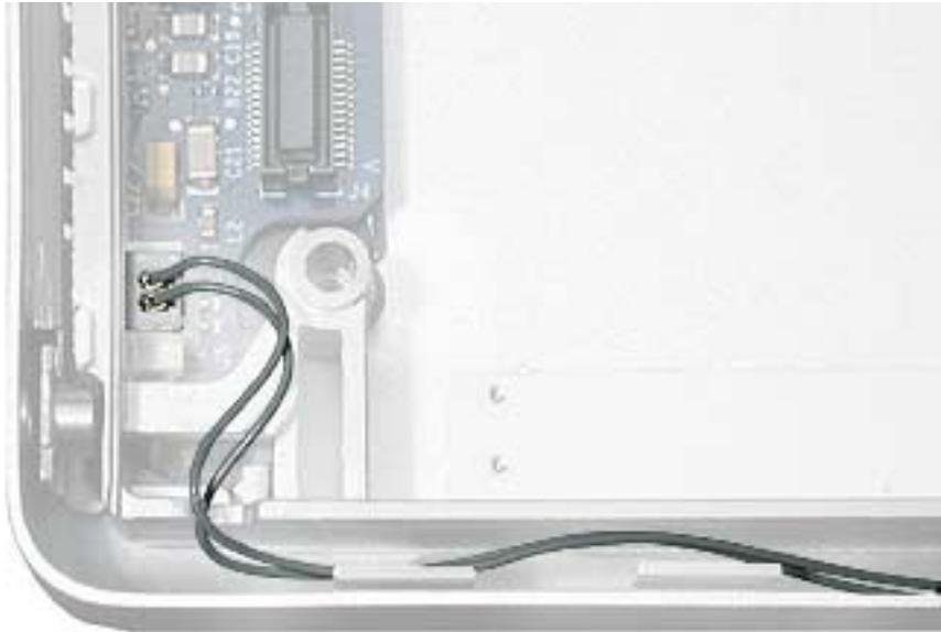
4. Install the replacement sound board, and reassemble the computer.
