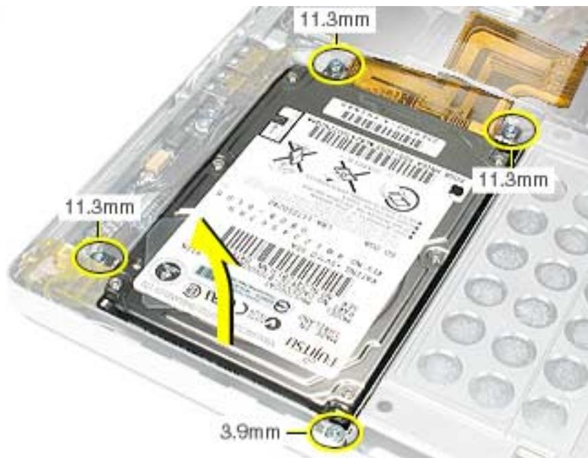
5. Transfer brackets, side screws, rubber shockpads and the flex cable to the replacement hard drive.
