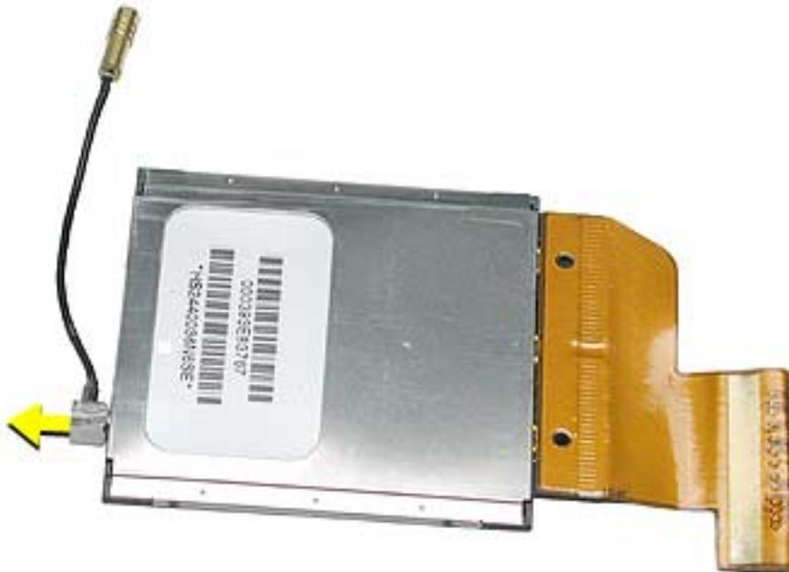
10. Install the AirPort Extreme card onto the PC card cage to be installed and reinstall the assembly.
