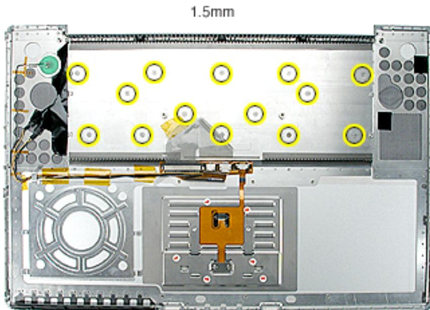
6. Start at the power button side and use a blunt tool (no wider than 3.5 mm) to carefully push on the keyboard screw bosses through the boss holes to begin to release the keyboard from its adhesive.
