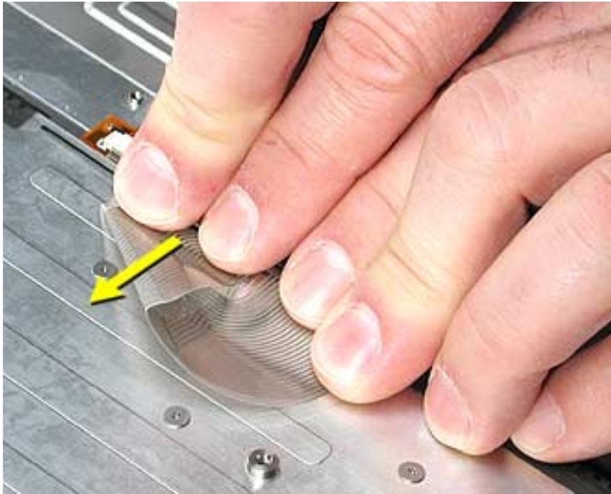
8. Use Kapton tape to secure the cable flat at the fold.
