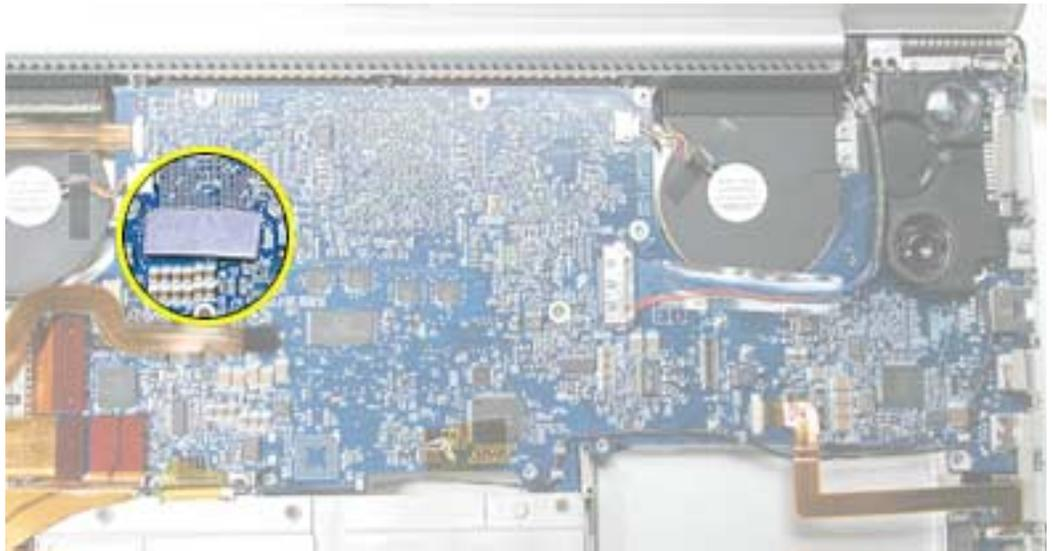
2. Visually check to verify that all cables (highlighted below) are connected and routed correctly with nothing raised up or incorrectly over a component.
