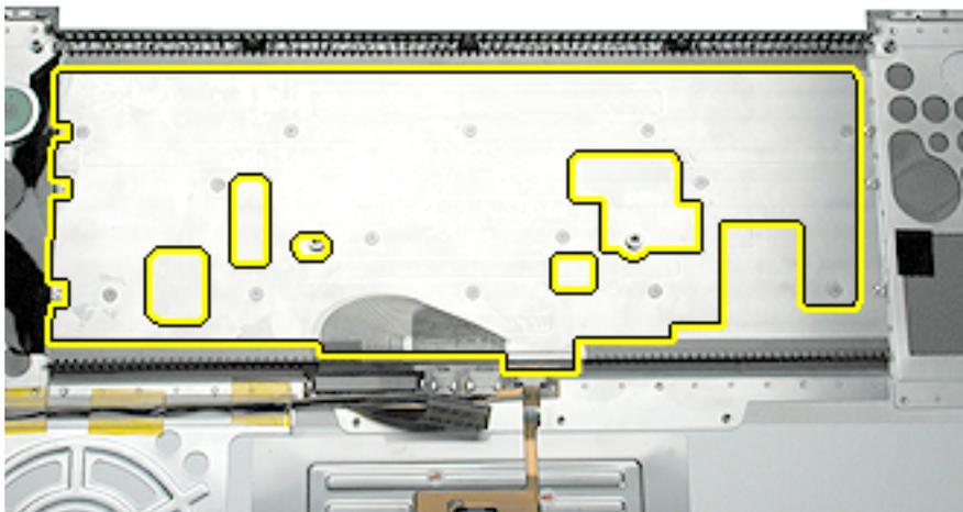
4. Remove remaining adhesive, if any, from the top case and screw heads.
