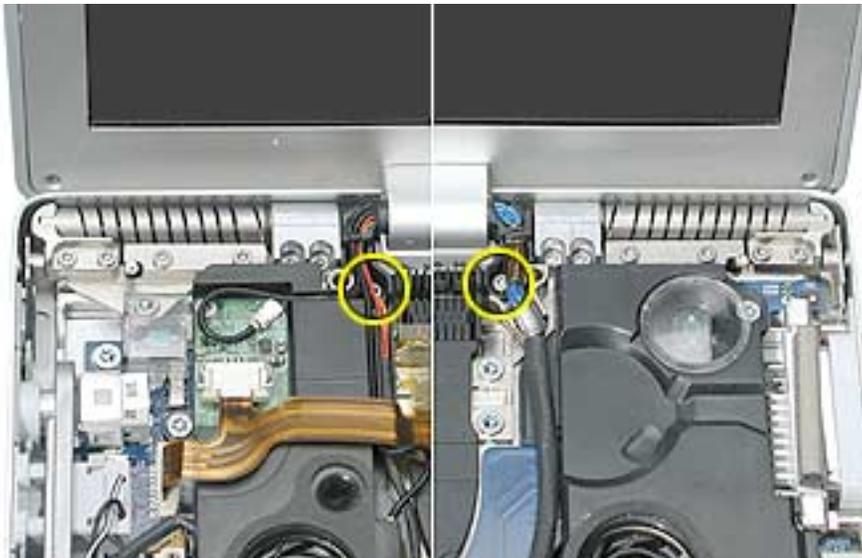
5. Move the display to a 90-degree angle and remove the two screws for the end caps of the clutch springs on each side.
