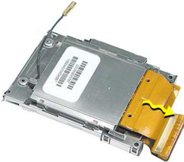
9. If replacing the AirPort Extreme card, pull the antenna jumper connector straight back to remove it. Transfer the cable extension to the replacement AirPort Extreme card.
