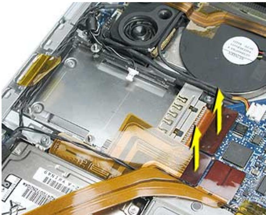
3. Pull out the coupling (joining the AirPort Extreme jumper and antenna cable) from the channel in the side of the left speaker. Grasp the coupling (not the wires) at both ends and pull to separate it at the middle.
