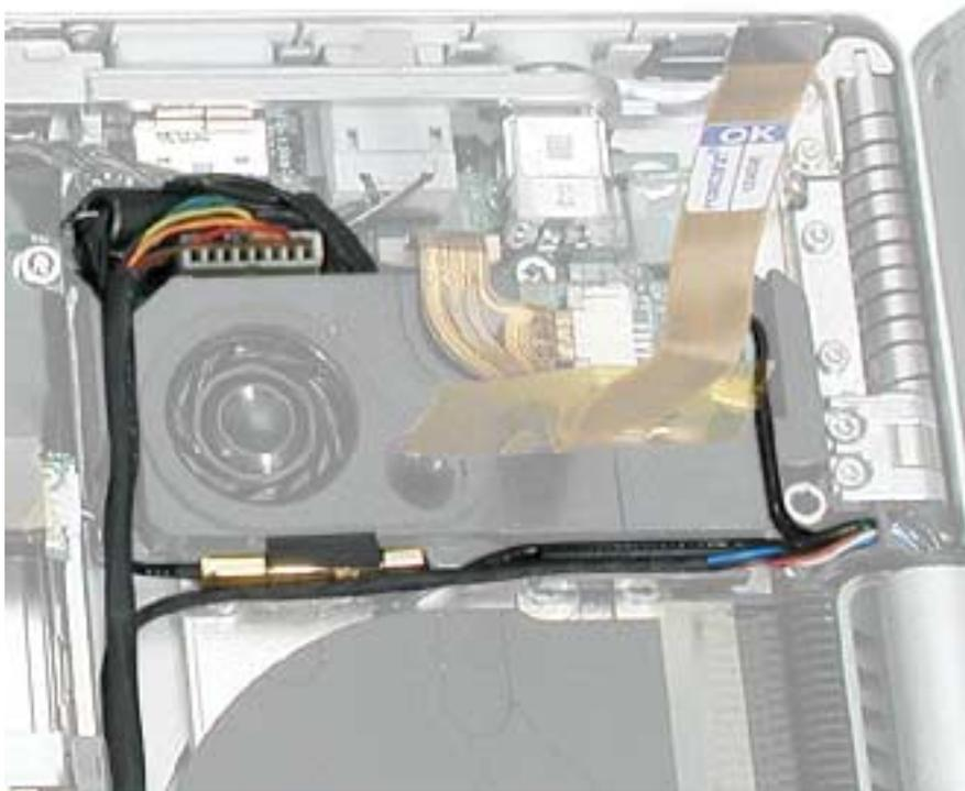
6. Verify that the LVDS cable's metal bead fits into the metal channel (rounded side up so that its teeth secure it) and that the cable is secured into the channel along the right speaker.
