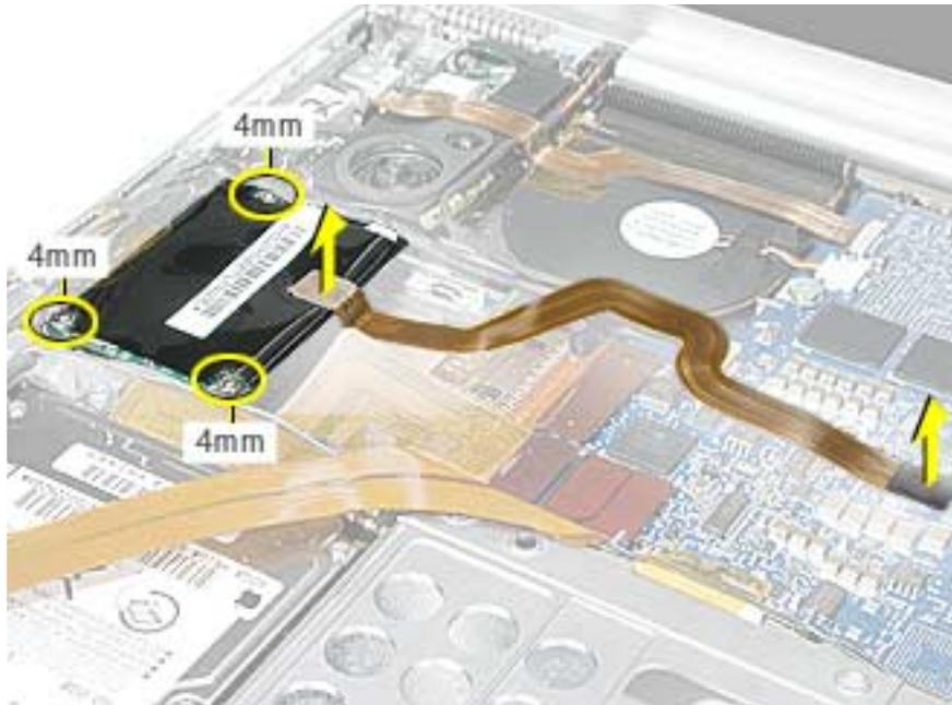
3. Lift the modem up slightly and disconnect the RJ-11 cable connector.
