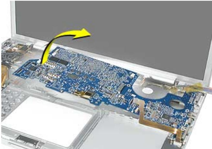
5. Carefully coax the port end of the board out of the port openings.
