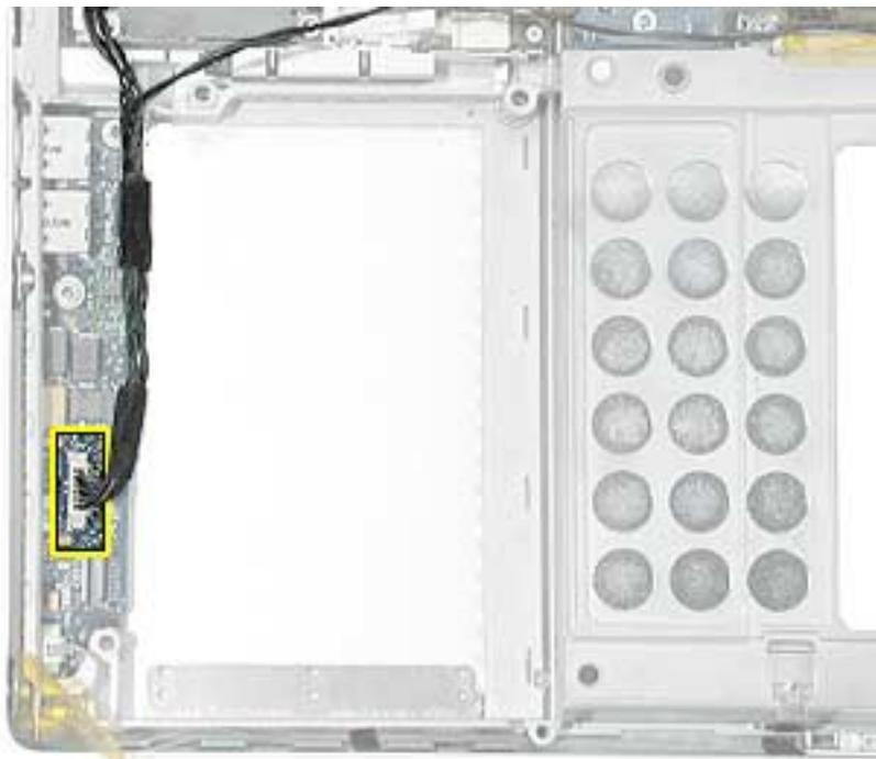
6. Install the replacement speakers, and reassemble the computer.
