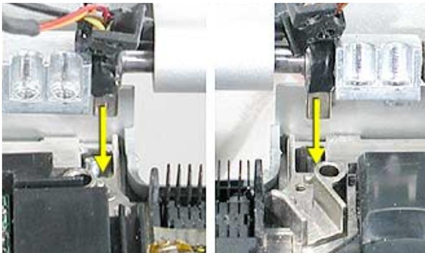
6. Install and tighten the screws for the clutch cleats, on both sides.
