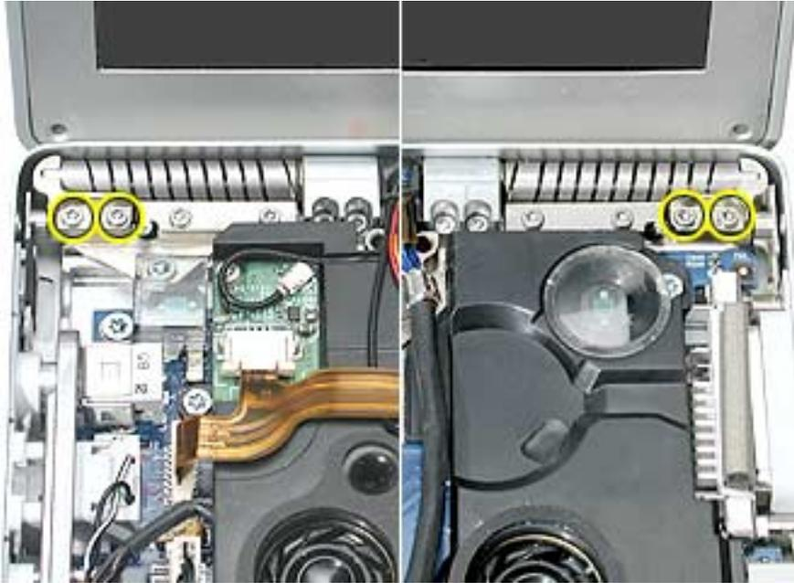
6. Remove the two clutch cleat screws on each side of the clutch barrel.
