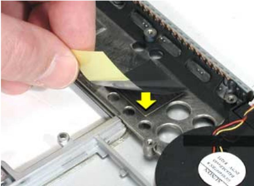
**Important:** With an X-Acto knife, trim any excess thermal pad material that extends beyond the mating surface, if necessary, to prevent it from touching holes in the heatsink.
