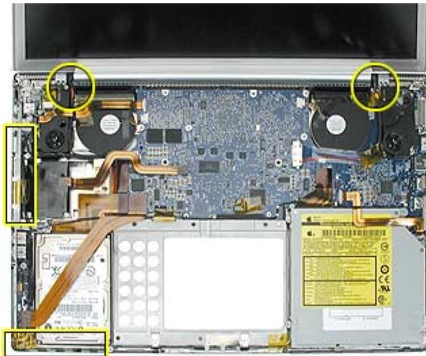
4. Check that display cable brackets are properly seated and secured with screws.
