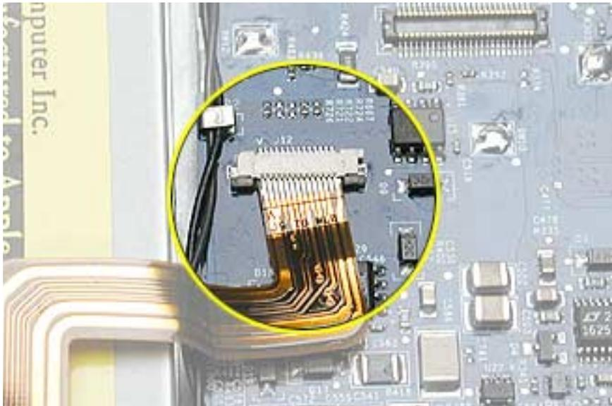
**Note:** If a cable is not securing properly, verify that it is inserted on the correct side of the locking bar.
