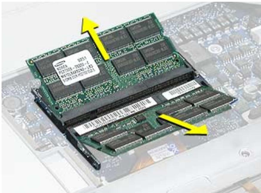
6. Align the notch in the board with the tab in the slot and insert the replacement memory cards at a 30-degree angle, pushing the card firmly until fully seated.
