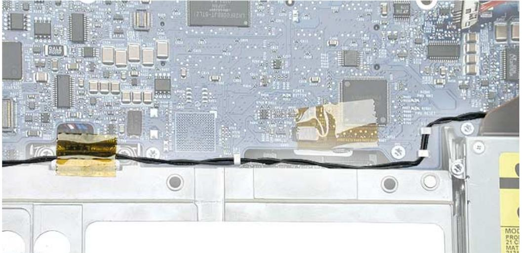
5. Disconnect the speaker wire connector from the sound board.
