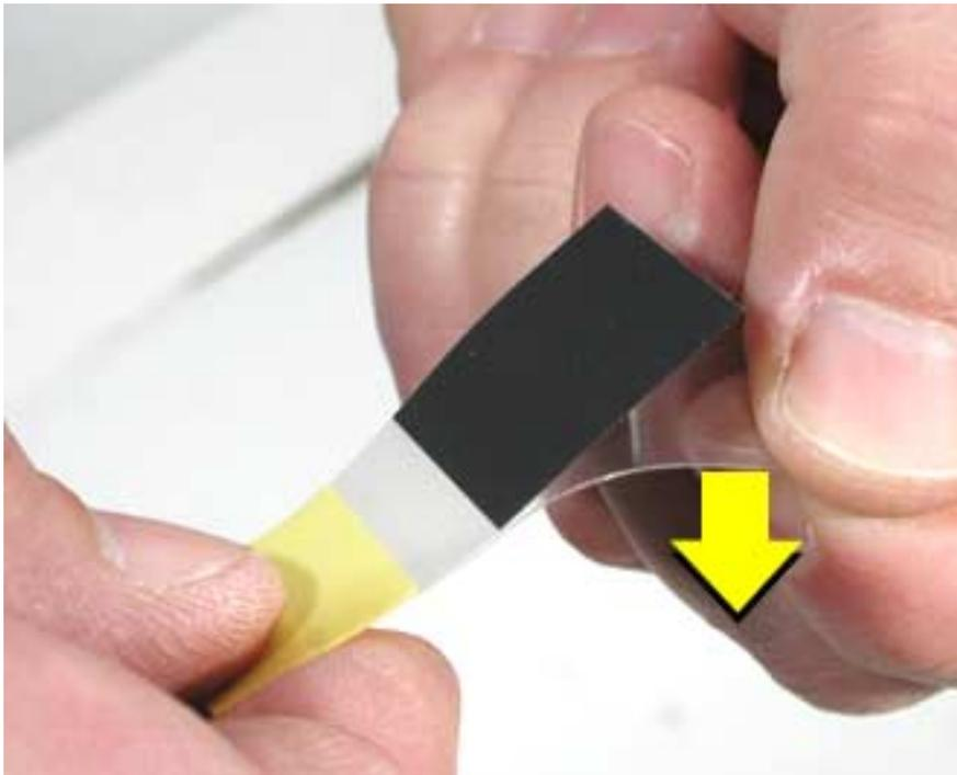
Center that side over the mating surface (raised surface) and evenly apply it, without air pockets, by lightly pressing on the protective backing of the other side.
