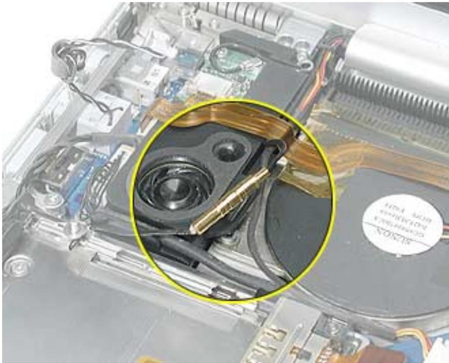
4. Remove two Phillips screws and two Torx T6 screws.
