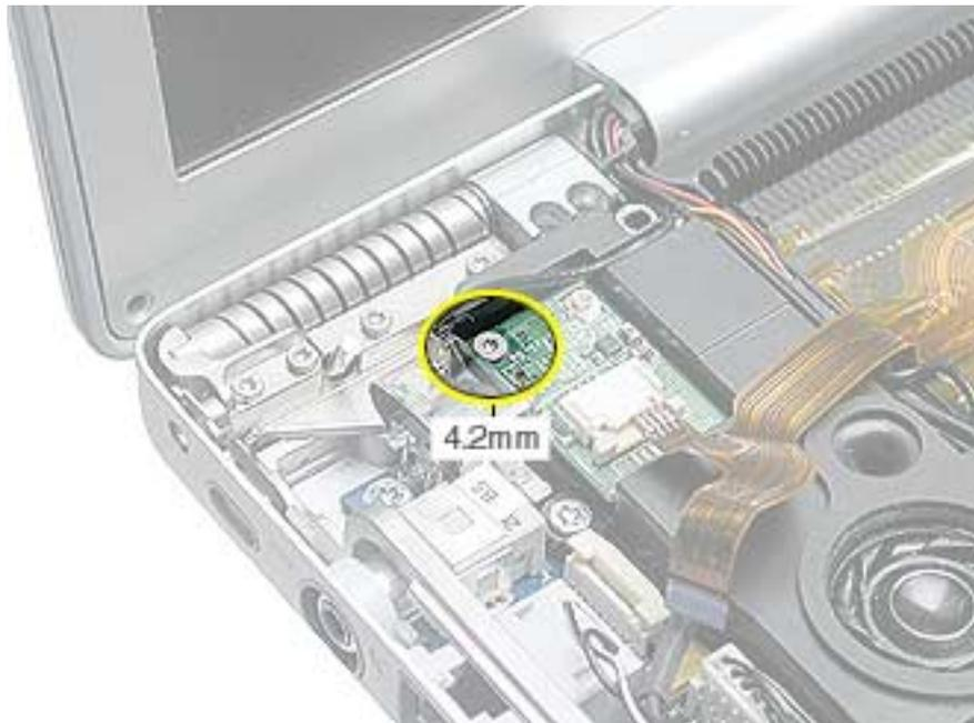
4. Install the replacement Bluetooth board, and reassemble the computer.
