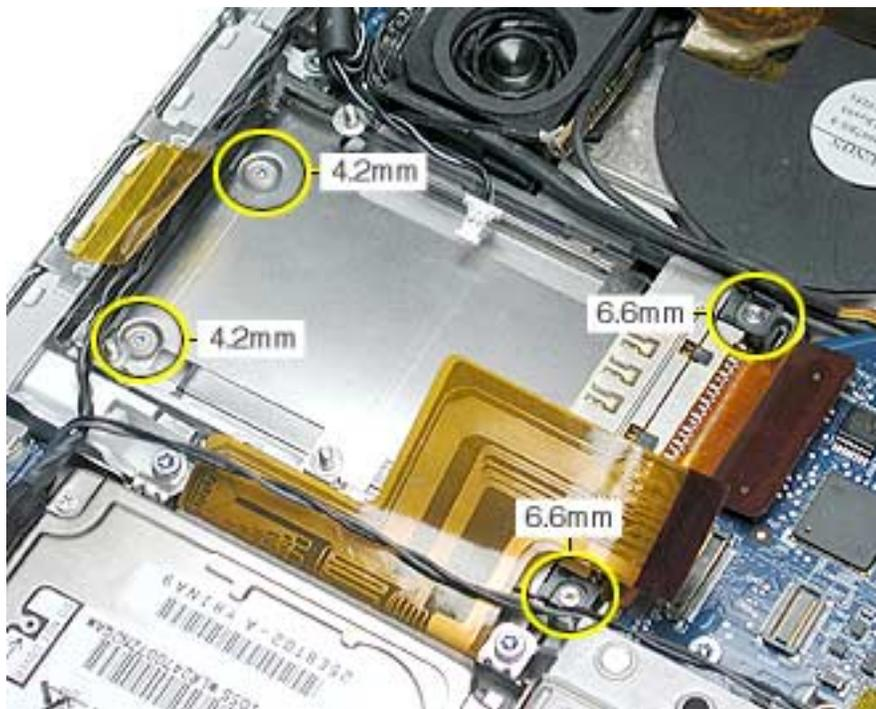
5. **Important:** The cross piece at the front end of the PC card cage is fragile. To avoid damage, do not touch this area while maneuvering the assembly.
