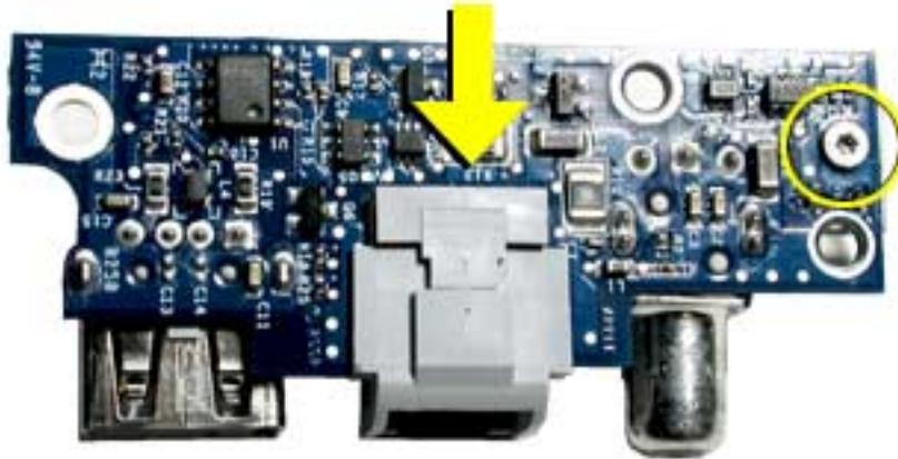
The ambient light sensor cover slides on and is attached with a screw from underneath the board.
