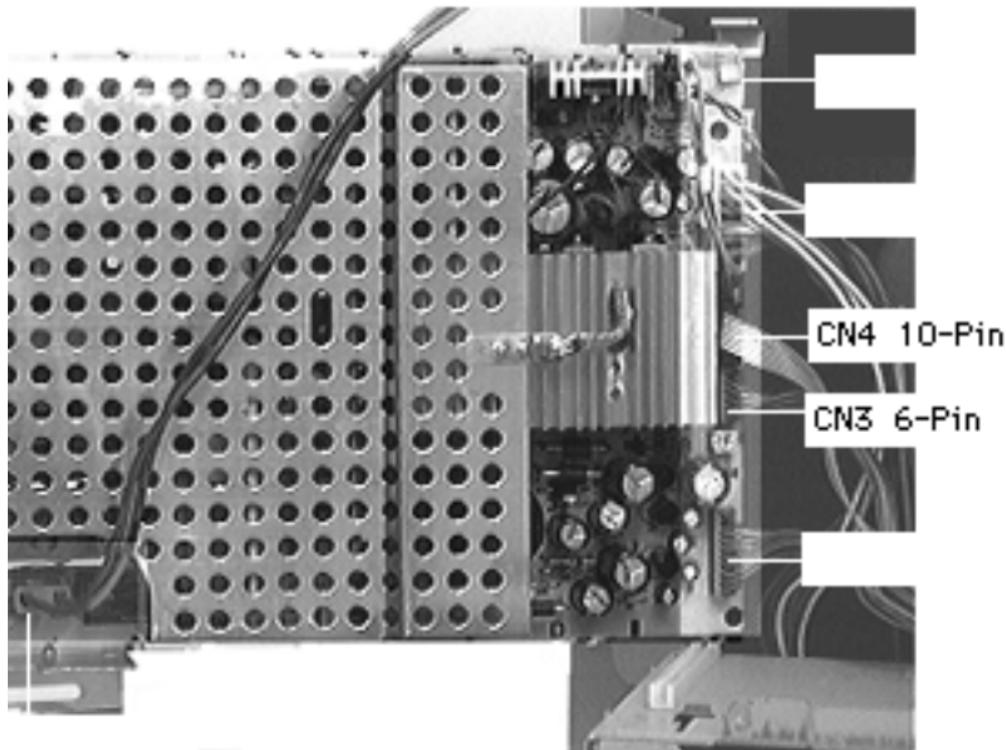
**Note:** The power supply-to-analog-board connectors are keyed and fit very tightly. You may need to use a jeweler's screwdriver to loosen the sockets of these connectors.
