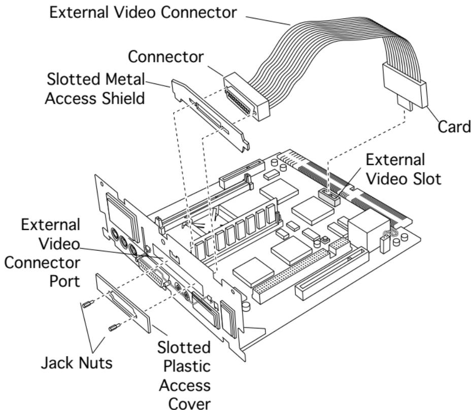
5 Insert the connector end of the ribbon cable through the slotted opening of the shield and fence.
