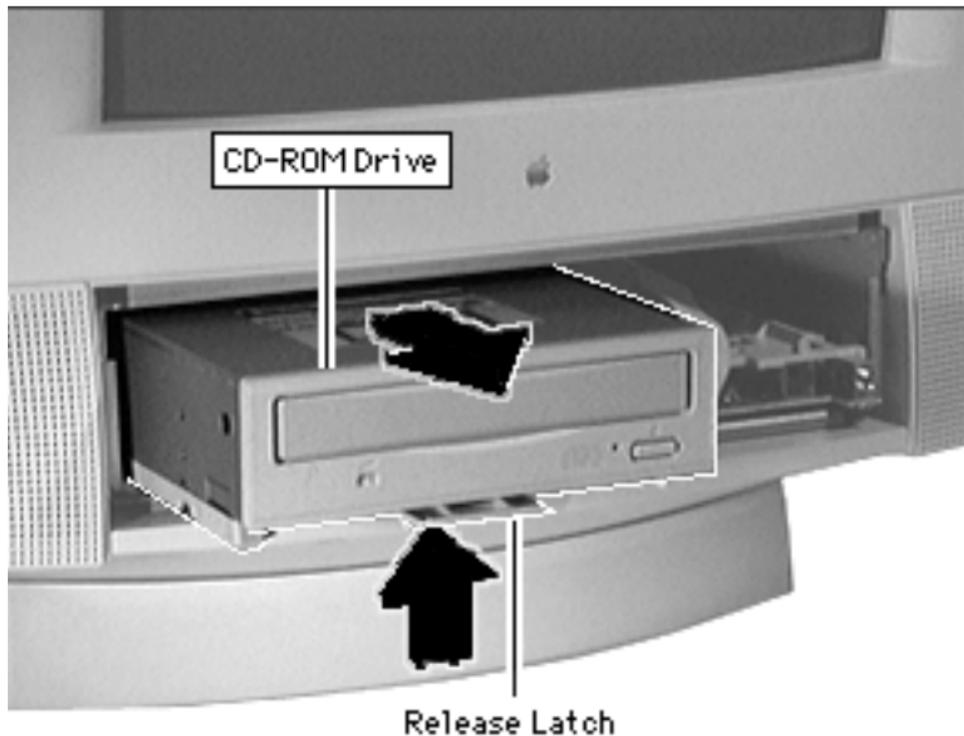
Push up the release latch and pull the CD-ROM drive from the chassis.
