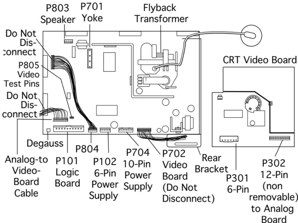
**Replacement Note:** This diagram shows the location of the rear bracket and the analog board cable connections:
