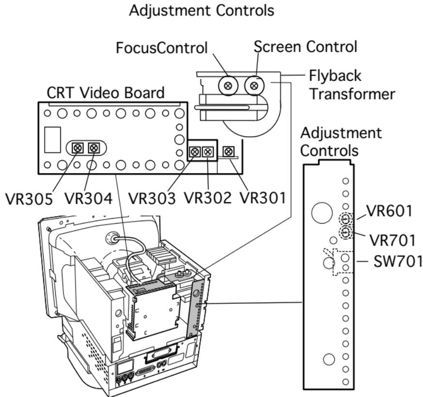
**Note:** The controls on this monitor require a small plastic Phillips-head tool or a small plastic flat-head tool to make adjustments.
