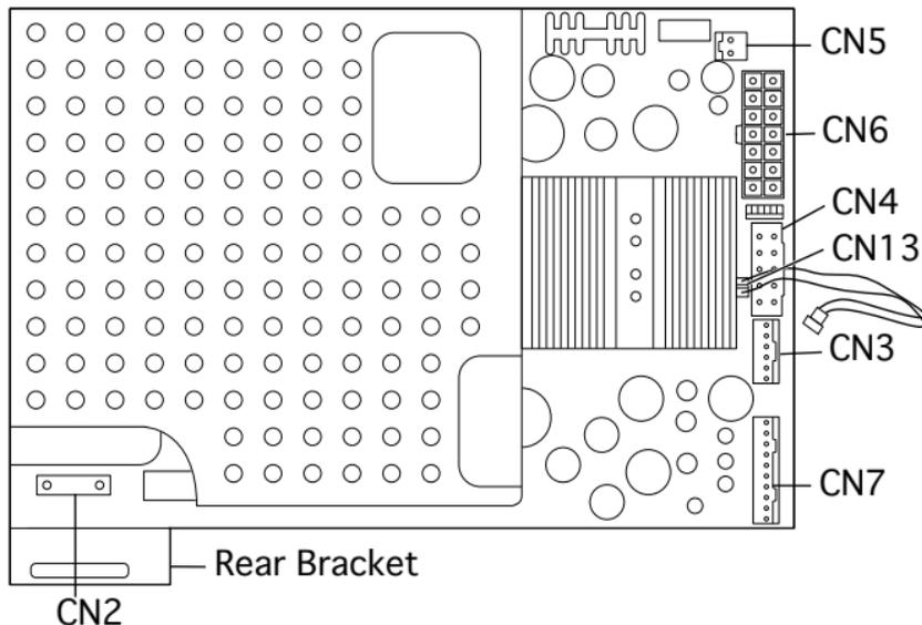
**Replacement Note:** This diagram shows the location of the rear bracket and the power supply cable connections for the original version. For Rev. B diagram, See “Power Supply, Rev. B”
