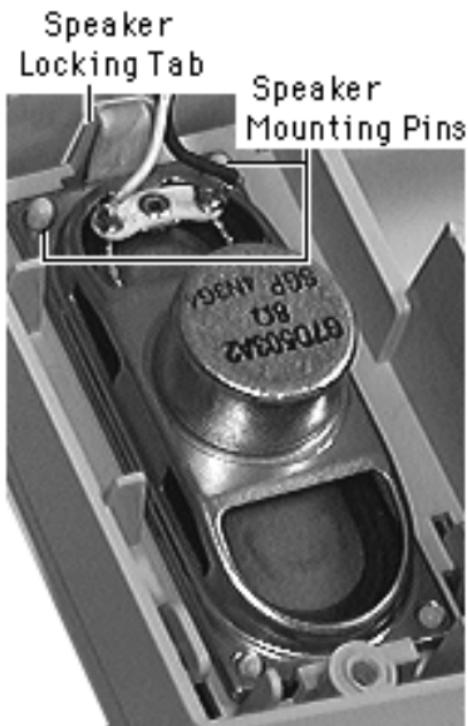
**Replacement Note:** Place the speaker with the longer cable on the floppy drive side of the unit. Align and secure the speaker with the bottom tabs inside the bezel. Then snap the top of the speaker over the two security pins.
