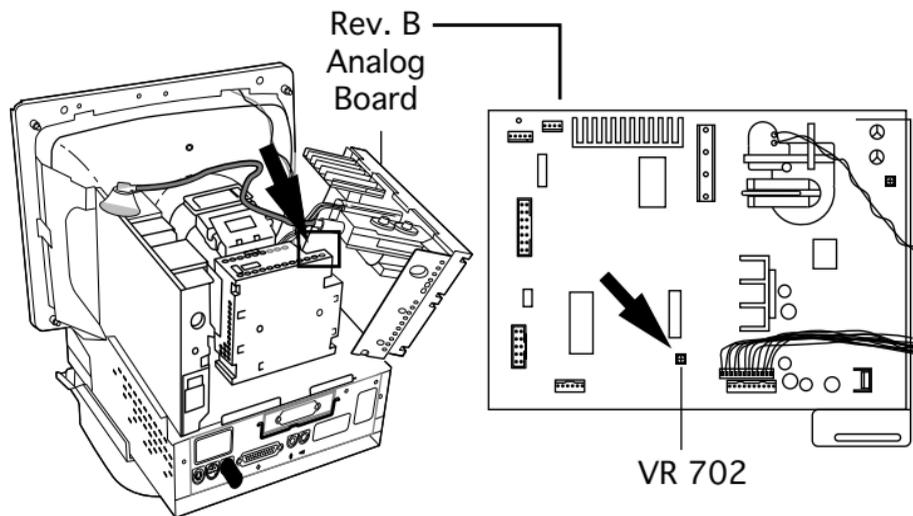
**Note:** To reach the VR702 high-voltage adjustment control on Rev. B computers, tilt back the analog board. The VR702 control is inside the analog board.
