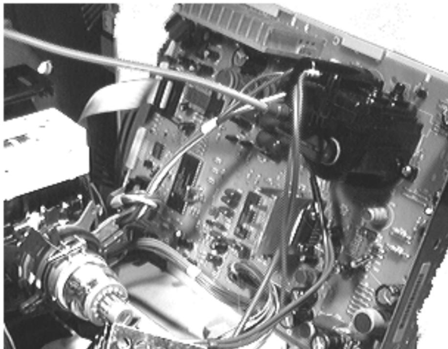
**Caution:** The analog and video boards of the two versions are not interchangeable. If you are servicing a Rev. B version, use the procedures in “Analog Board, Original Version” and substitute the following cable locations.
