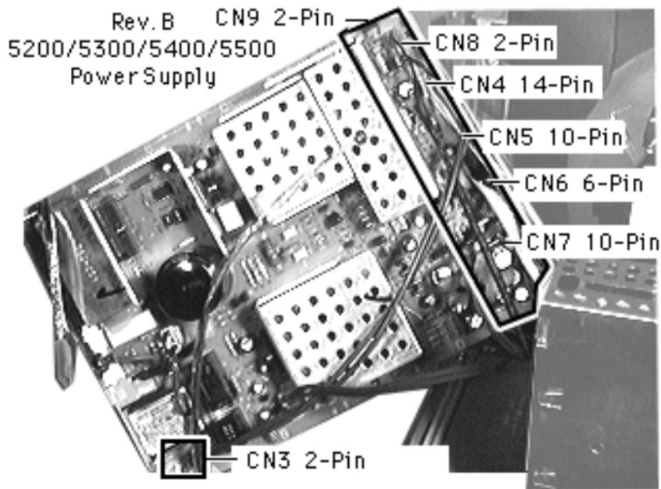
you are servicing an original version, use the procedure in “Power Supply, Original Version.”
