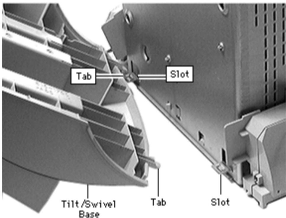
**Replacement Note:** Align the tabs at the front of the tilt/swivel base with the slots in the chassis. Angle the tilt/swivel base and slide in the tabs.
