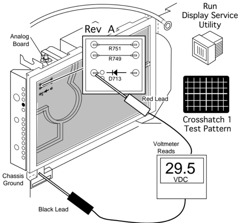
**Replacement Note:** Perform the high voltage adjustment whenever you replace the CRT or the deflection board.
