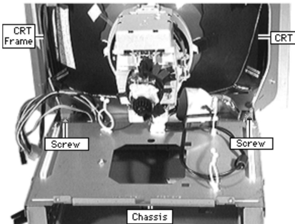
**⚠ Warning:** Support the top of the CRT. The CRT is very heavy and may fall forward as you complete this procedure.
