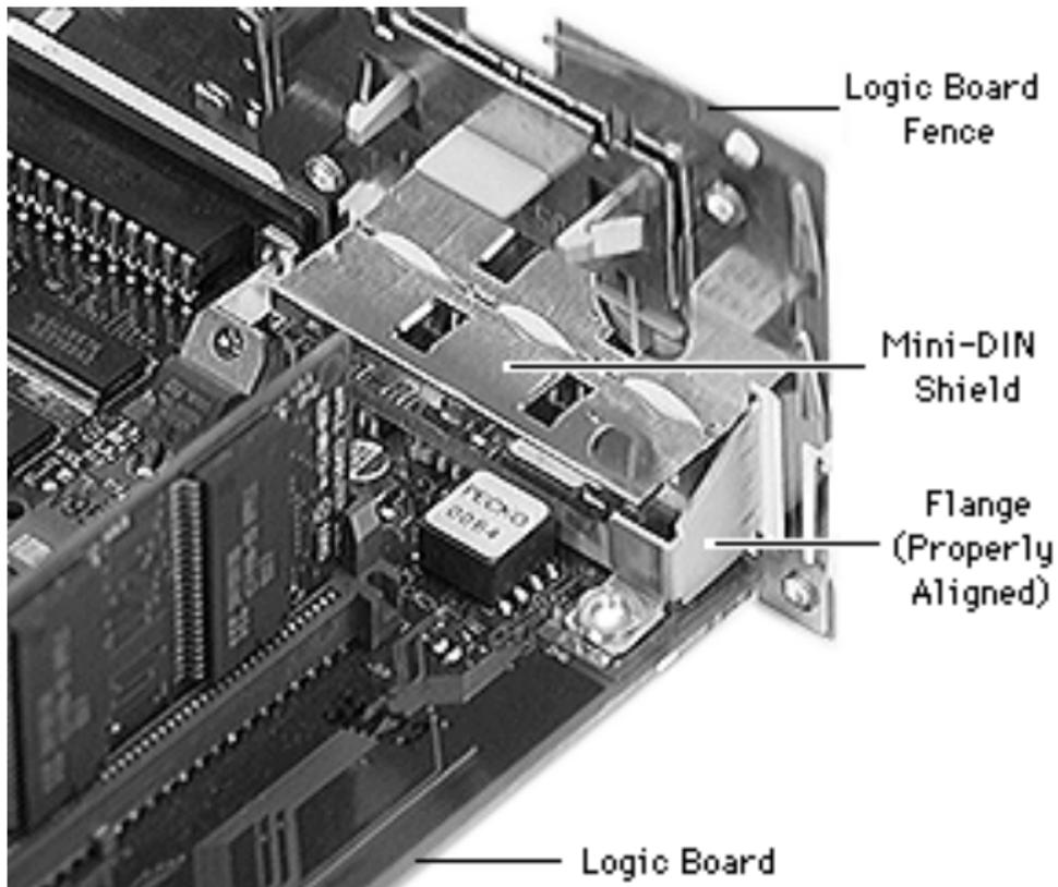
**Replacement Note:** Verify that the flange on the logic board fence is properly aligned with the mini-DIN shield.
