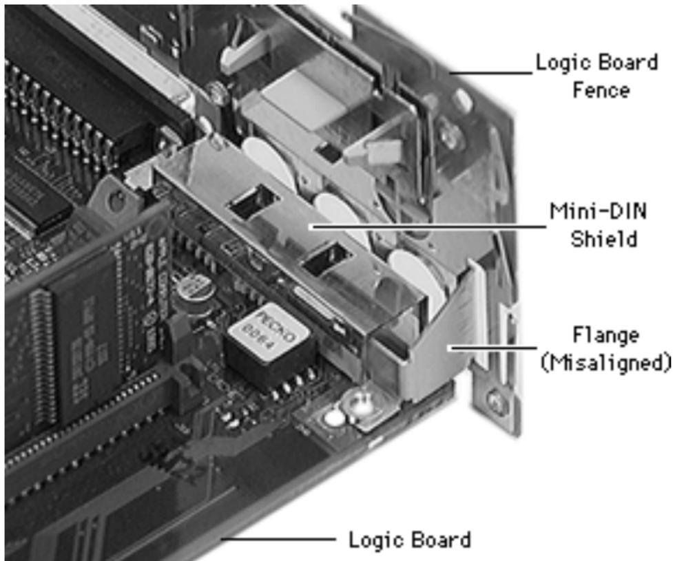
Align the flange around the mini-DIN shield first, then swing the rest of the logic board fence into place.
