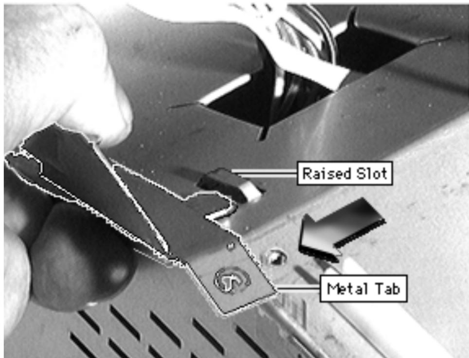
**Replacement Note:** Align the line of tabs on the CRT frame with the line of slots on the front of the chassis.
