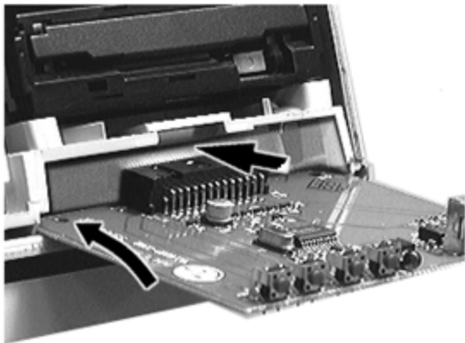
**Replacement Note:** Tilt the board up slightly to insert it into the guide rails.
