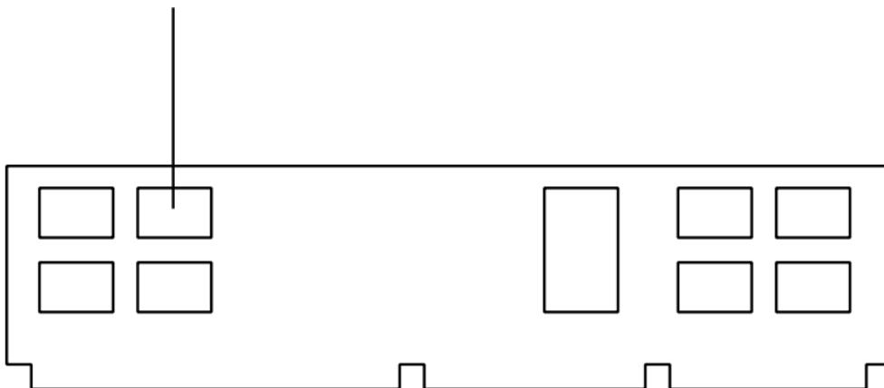
If this number, not counting the Q or any other letters present, has four digits, the cache is incompatible with an OPC logic board. Replace this L2 cache DIMM with part number 661-1477.
