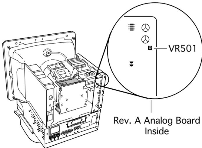
**Note:** The VR501 control is inside the analog board.
