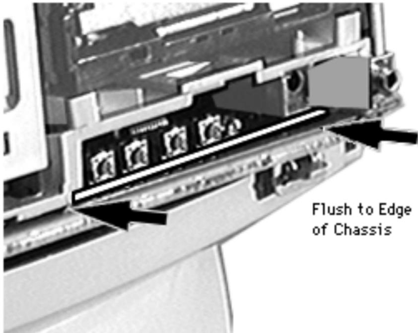
**Replacement Note:** The front edge of the reinstalled front-panel control board must be flush with the front edge of the plastic chassis.
