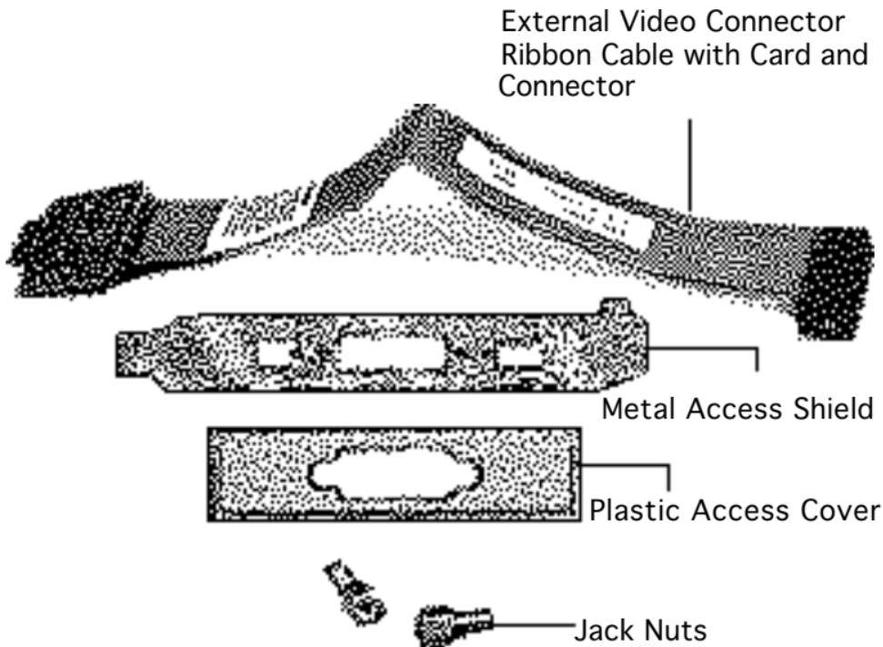
**Note:** The Apple External Video Connector provides “mirroring” or display of the system’s monitor screen on a presentation screen. In addition to the ribbon cable with card and the connector, the Apple External Video Connector kit includes a metal access shield, a plastic access cover, and two jack nuts.
