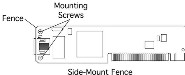
**Replacement Note:** If you are installing an Ethernet card and its fence does not include a hook, replace the fence.
