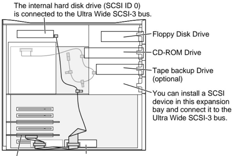
One 5.25" Hard Disk Drive or two 3.5" Hard Disk Drives can be installed on the floor of the server and connected to the Ultra Wide SCSI-3 bus. (Some Workgroup Server models come with a second Hard Disk Drive [SCSI ID 1] installed here.)
