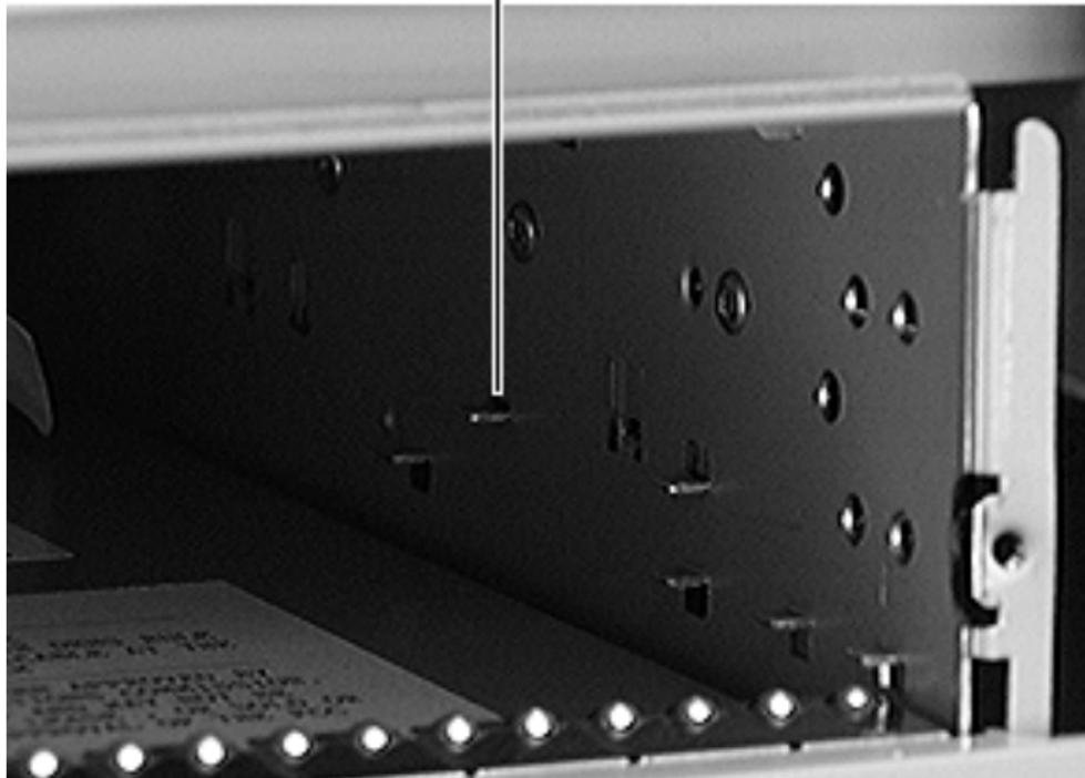
**Replacement Note:** When inserting the drive into the computer, make sure the drive carrier aligns with the carrier guides. The carrier should slide between five metal tabs below and two metal tabs above the left and right edges of the carrier.
