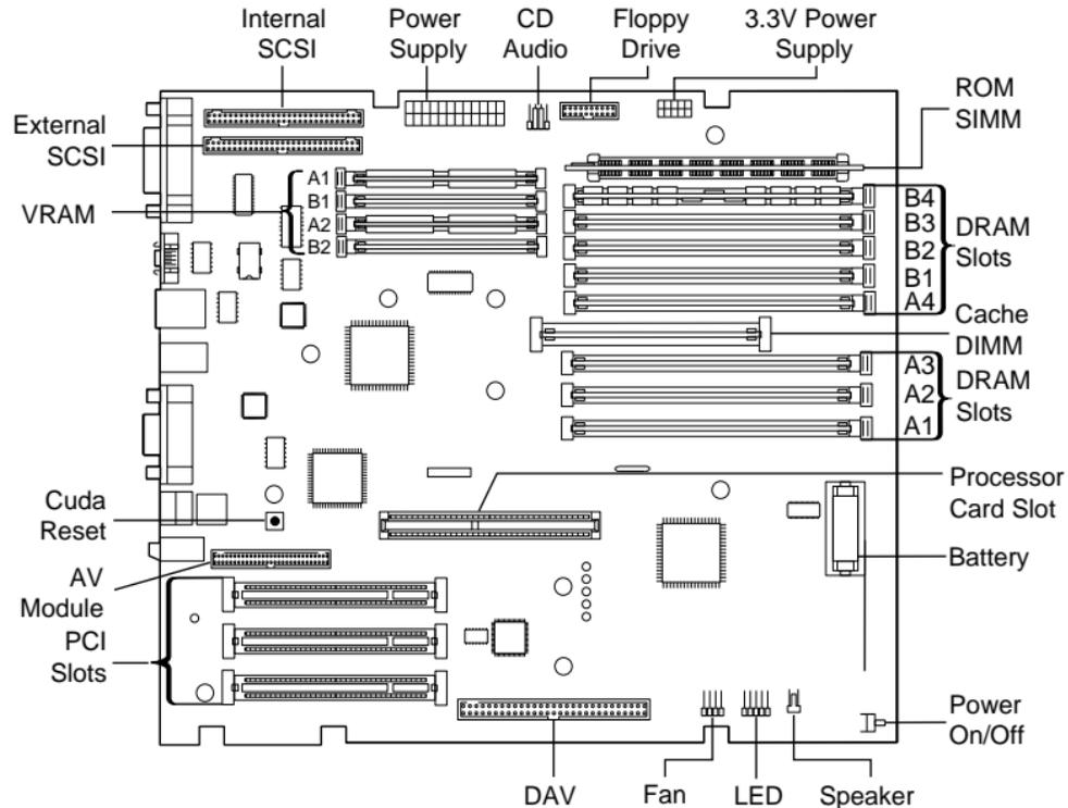
Figure: PM 8600/200 Logic Board
