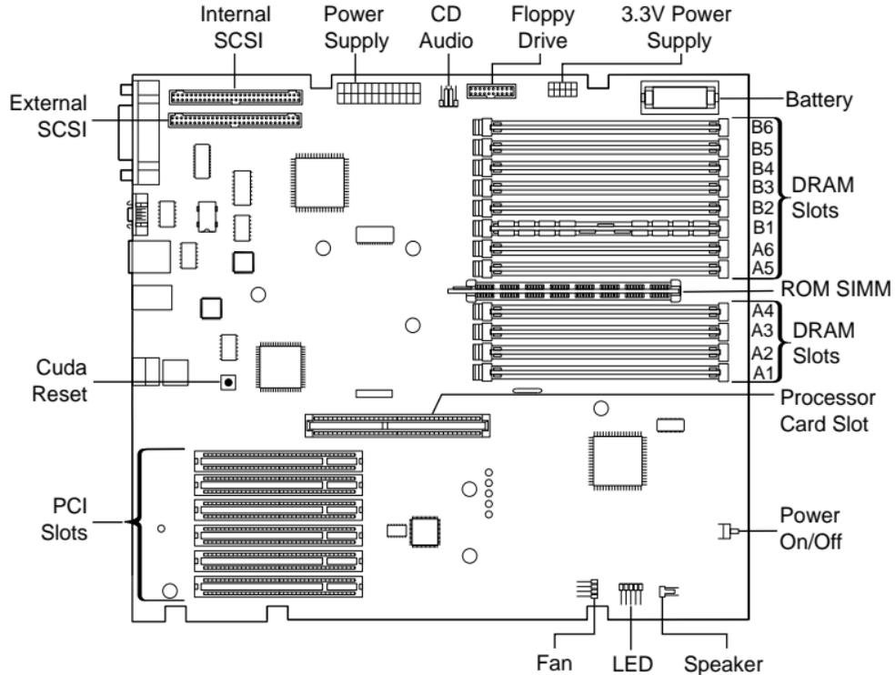
Figure: PM 9600/WS 9650 Logic Board
