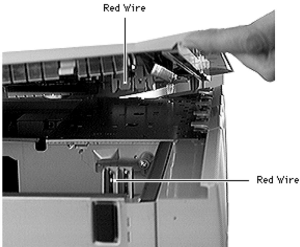
**Replacement Caution:** Make sure the red fan cable wire in the speaker housing matches up with the red fan cable wire in the side access panel.
