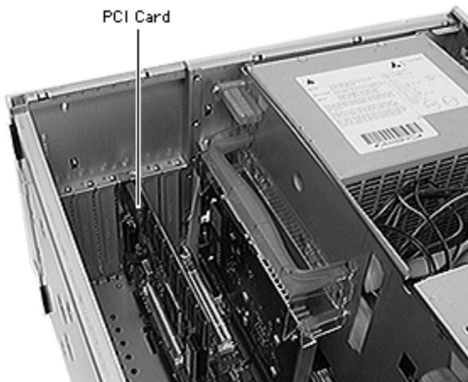
**Note:** This procedure explains how to install a PCI card.
