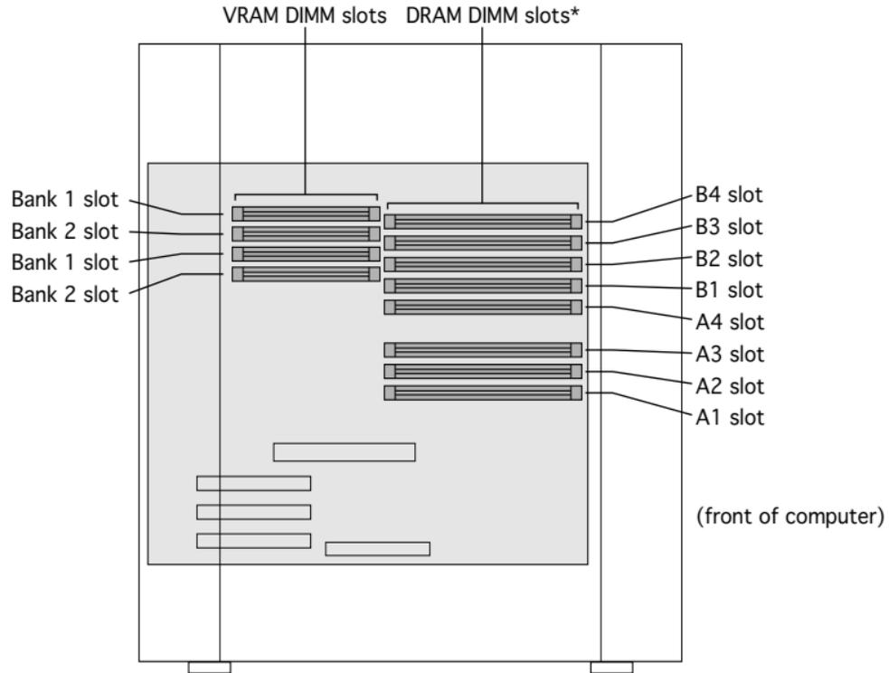
**Figure: PM 8600 Series DRAM DIMM Slots**
