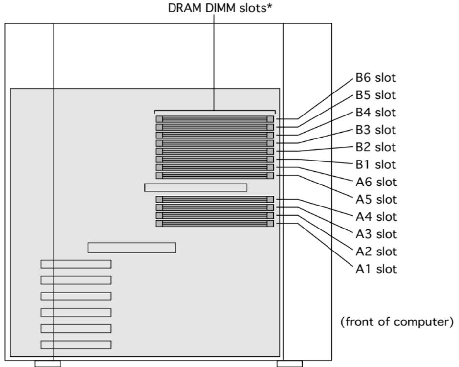
**Figure: PM 9600/WS 9650 DRAM DIMM Slots**
