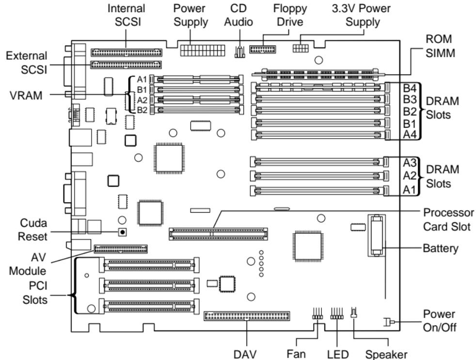
Figure: PM 8600/250 & 8600/300 Logic Board
