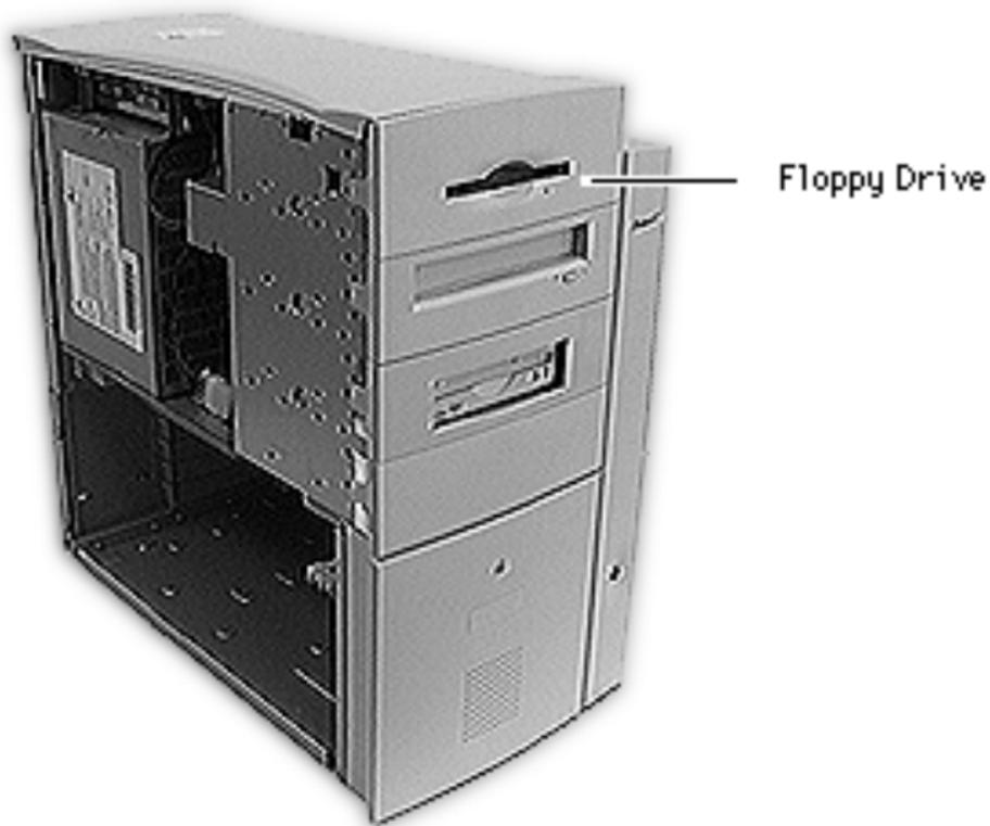
**Note:** This topic includes instructions for removing the floppy drive bezel, floppy drive shield, front drive carrier, and floppy drive.
