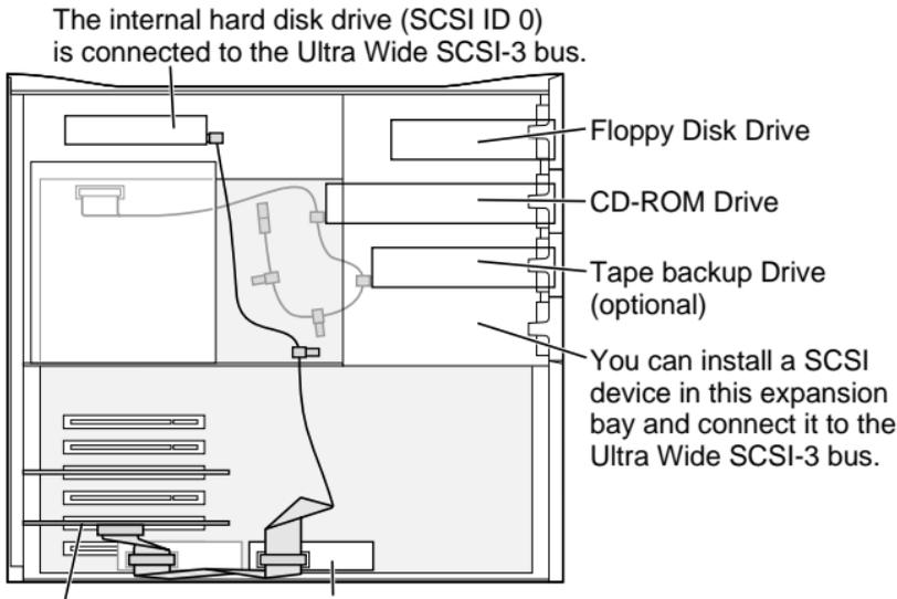
**Replacement Note for WS 9650 Only:** Depending on what type of drive you install (50-pin or 68-pin) you will need to connect either the 50-pin SCSI cable or the Ultra Wide SCSI cable to the drive. The graphic at left shows the routing of the two SCSI cables in the WS 9650.
