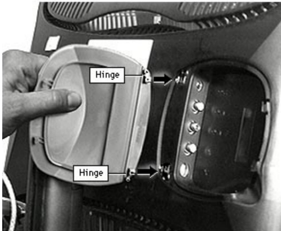
**Replacement Note:** Align the two hinges on the A/V door to the two small openings on the rear housing. Press the A/V door into place.
