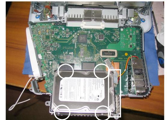
5. Remove four screws holding hard drive into bracket. Disconnect power and connector cables.
